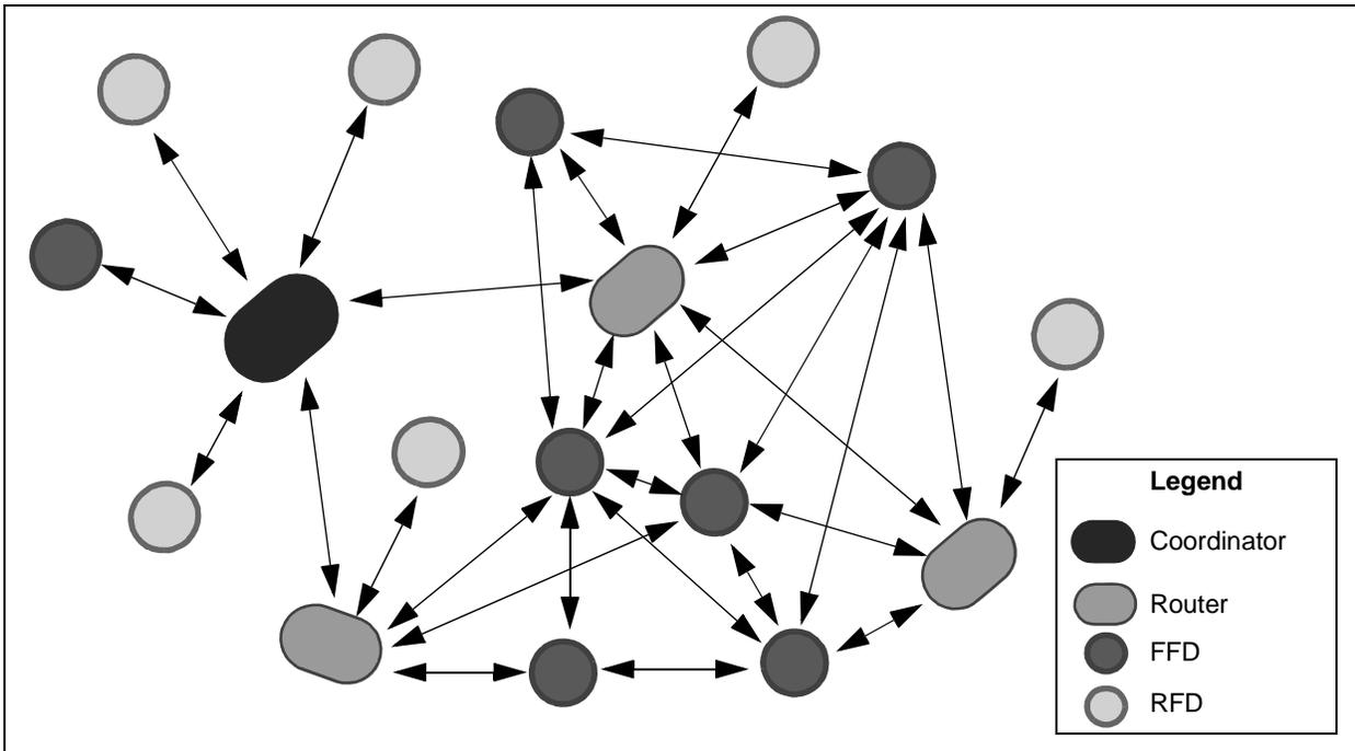
The cluster tree and mesh topologies are also known as multi-hop networks, due to their abilities to route packets through multiple devices, while the star topology is a single-hop network. A ZigBee protocol
