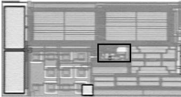
Figure 6. Die photograph of current source including startup circuit.
