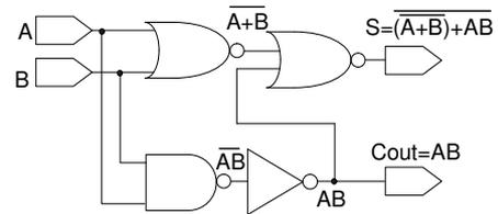
Fig. 3 Half adder which consist of NOR, NAND and NOT logic.
