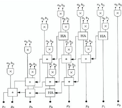
Fig. 2 Details for a 4x4 array multiplier.
