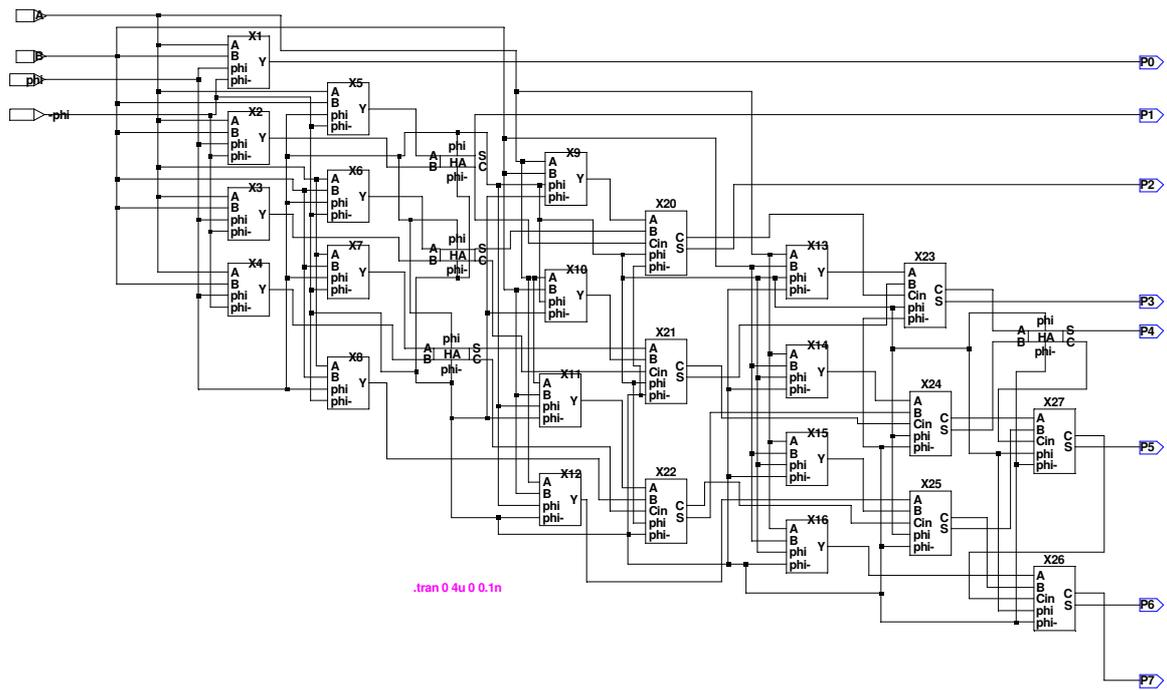
Fig. 5 4x4 array multiplier block diagram.
