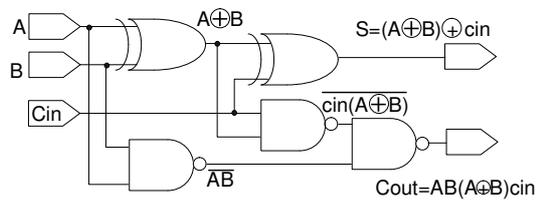
Fig. 4 Full adder which consist of XOR and NAND logics.
