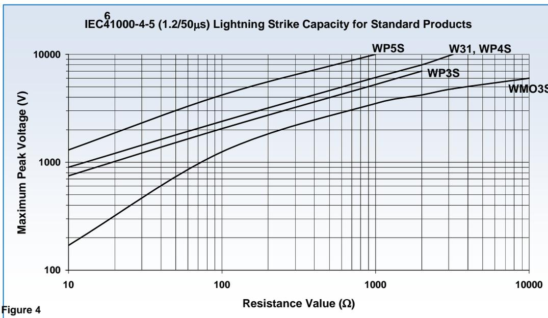
When calculating the peak voltage across the line input resistor it is necessary to subtract the clamping voltage of the MOV, typically 700 to 1000V, from the peak voltage applied to the circuit.
