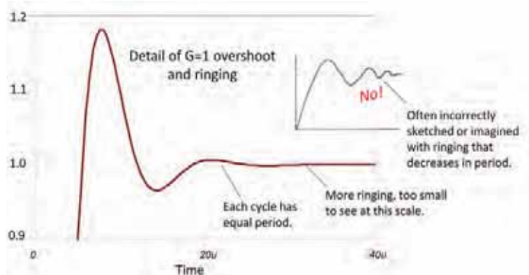
Figure 55: An expanded view of a G = 1 small-signal showing that the period of ringing is constant.
