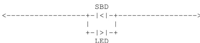
The LED is soldered close to SBD using as short of leads as possible (being careful not to ruin either part with too much heat). (Note that the diodes are connected anode to cathode, not cathode to cathode.)
