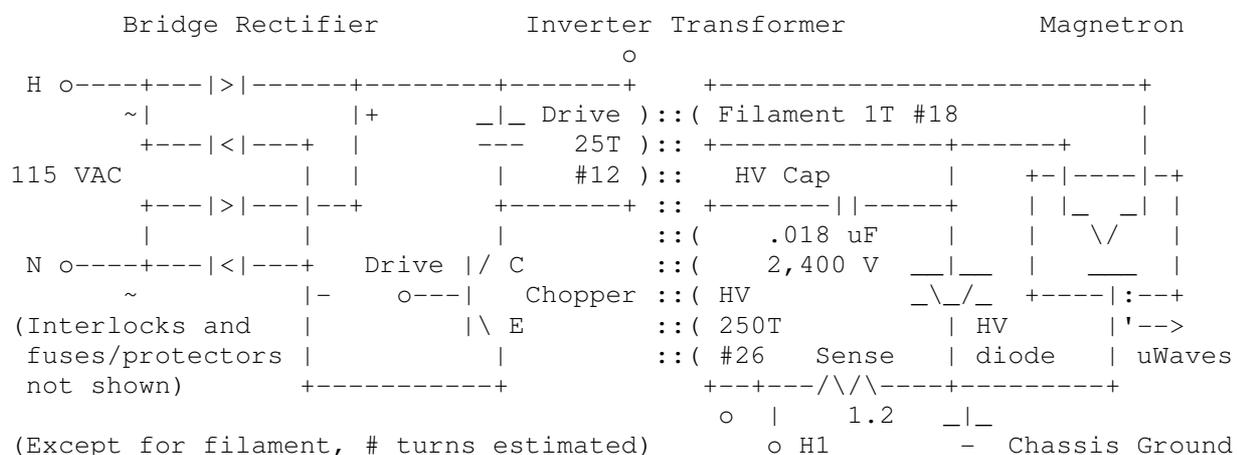
The chopper transistor is marked: Mitsubishi, QM50HJ-H, 01AA2. It is a LARGE NPN type on a LARGE heatsink. :-)
