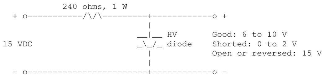
The voltage drop in the forward direction should be at least 6 V with a few mA of current but may be somewhat higher (8 V or more) with a few hundred mA. If your DMM or VOM has a resistance scale operated off a battery of at least 6 V, you may get a reading in one direction (but only one) without the need for an external power supply.
