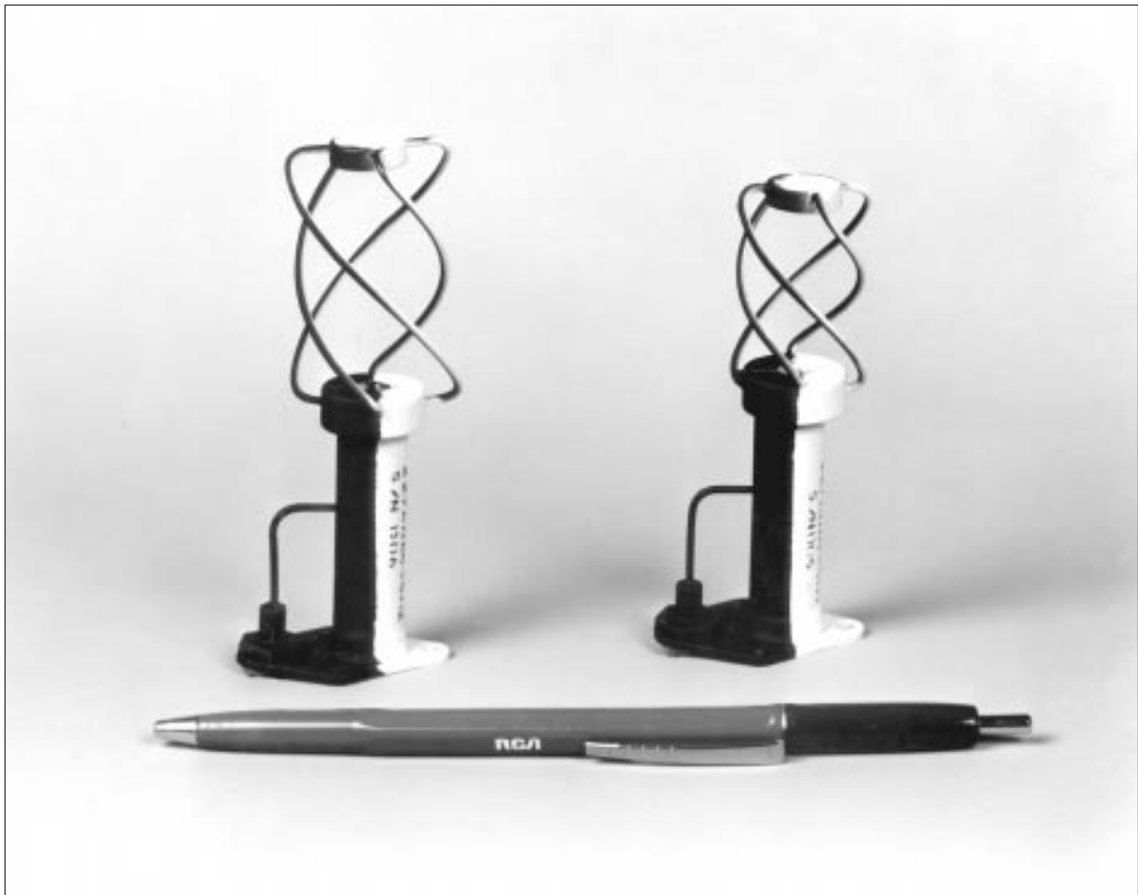
Fig 22-1 — Two flight-model quadrifilar helix antennas. The larger is for use around 1800 MHz, and the smaller around 2200 MHz. Radiation from each antenna is circularly polarized and of the same screw sense everywhere throughout its radiation sphere.
