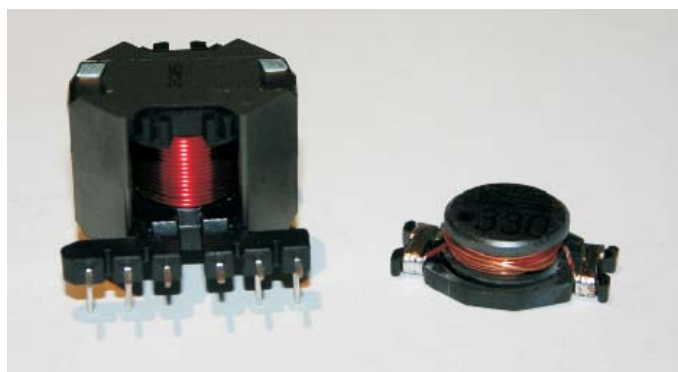
Figure 2: (a) 47 \mu\text{H} custom inductor and (b) off-the-shelf commodity component.
