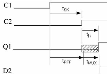
$$t_{SK} \leq \min t_{PFF} - t_h$$
