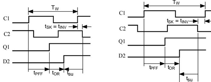
C2 skewed after C1:  $T_W \geq \max T_{PFF} + \max t_{NET} + t_{su} - \min t_{INV}$
