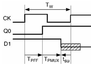
$$T_W \geq \max t_{PFF} + \max t_{PMUX} + t_{su}$$
