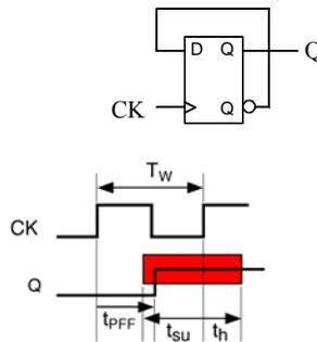
$$T_W \geq \max t_{PFF} + t_{su}$$
