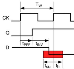
$$T_W \geq \max t_{PFF} + \max t_{PINV} + t_{su}$$
