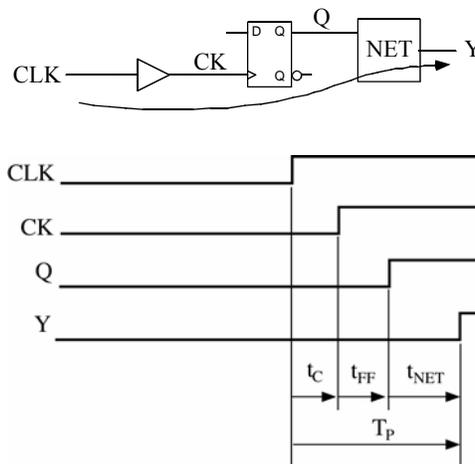
$$T_P = t_C + t_{FF} + t_{NET}$$
