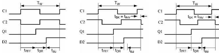
$$T_W \geq \max T_{PFF} + \max t_{OR} + t_{su}$$
