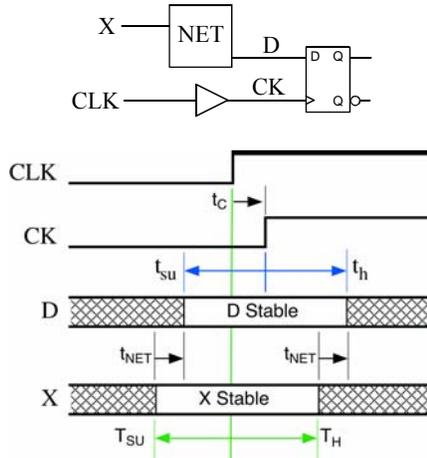
$$T_{SU} = t_{su} + \max t_{NET} - \min t_C \quad T_H = t_h - \min t_{NET} + \max t_C$$
