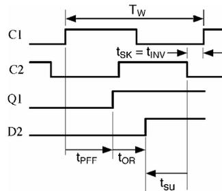
$$T_W \geq \max T_{PFF} + \max t_{OR} + t_{su}$$
