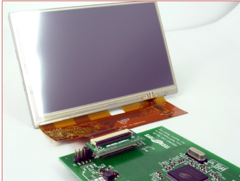
Figure 2.2.0 Connect 5" TFT to SSD1963EVK
