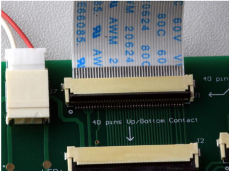
Figure 4.3 Connection of J1 and J7 for 7" TFT panel (TY700TFT800480)
