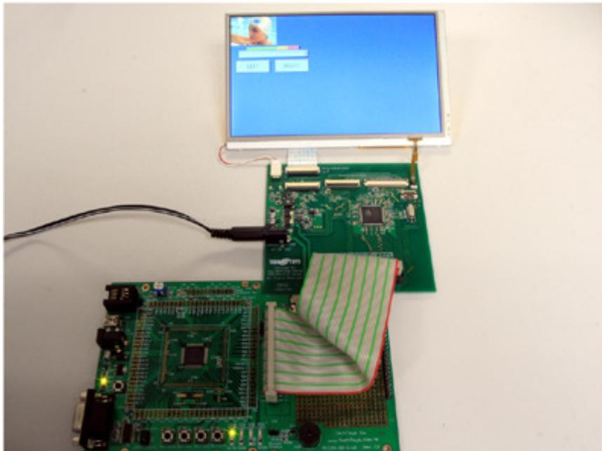
**Figure 6.3** PIC24/32 Eval with PIC32MX running Microchip Graphic Library Version 2.00 on a 7" TFT
