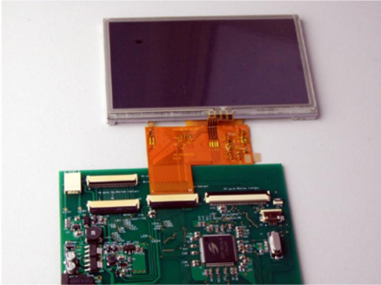
**Figure 4.5** Connect 4.3" TFT panel TY430TFT480272 to J3
