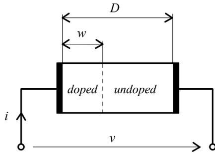
Fig. 1. Memristor model according to [1].
