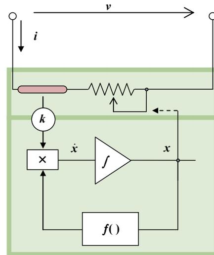
Fig. 3. Block diagram of the memristor model.
