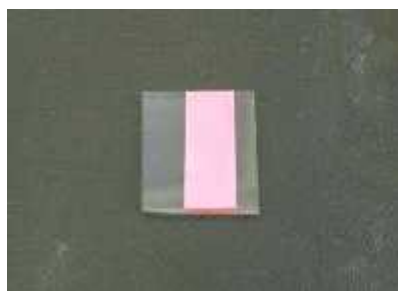
Fig2.5: ITO dipped in dye solution
