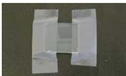
Fig2.1: masking of ITO Glass
