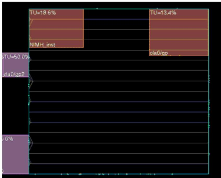
The following figure illustrates the result with you use the `flattenPartition` command with the `-bringbackRow` parameter. In this case, the NIMH rows and the unaligned rows are brought back to the top-level inside the power domain.
