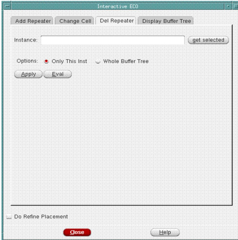
2. Enter the buffer instance name to be removed in the *Instance* field.
