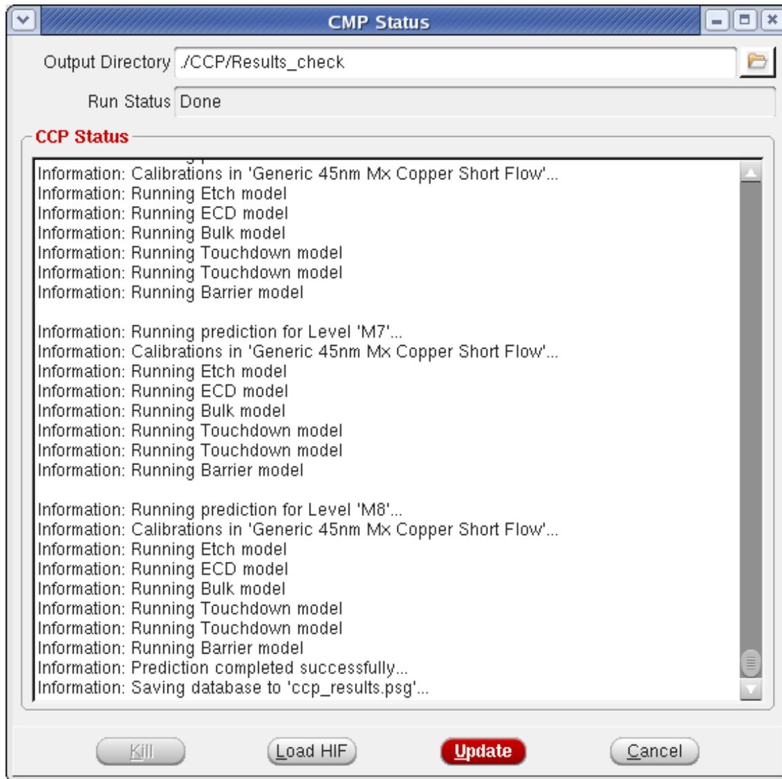
On completion of the CMP run, the *CMP Status* window displays the summary of the hotspots detected by the run and an `rdB` format output file is generated in the results directory.
