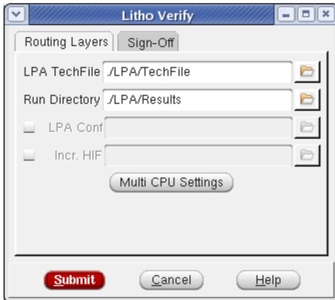
3. In the *Run Directory* field, specify the LPA output directory that will contain one subdirectory for each layer (POLY, M1, etc.) when LPA is run with the configuration file for that layer.
