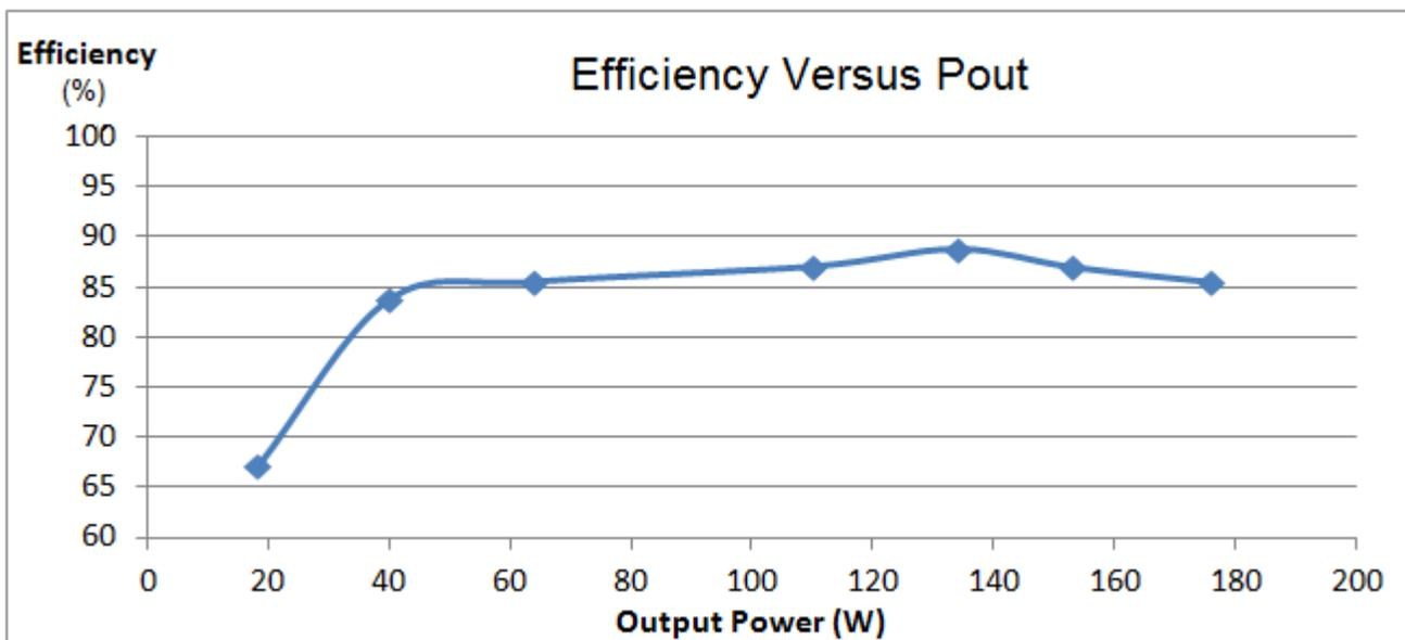
Figure 5. Efficiency Curve with Respect to Output Wattage
