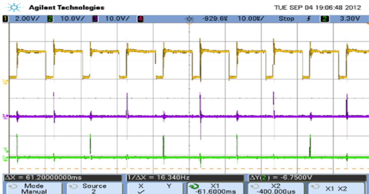
Figure 3. MSP430 Clock Output (Channel1) and Gate Drive for each MOSFET at No Load
