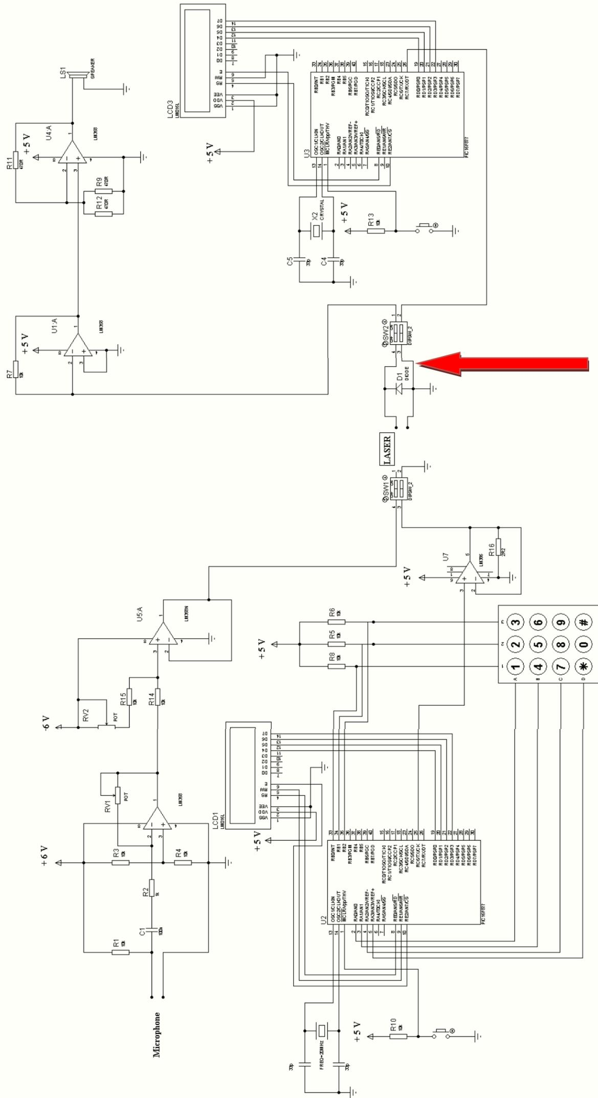
The photodiode is connected to the UART Rx terminal directly. Its not working actually. Can anyone suggest an intermediate circuit in between photodiode and Microcontroller Rx terminal for proper UART signal reception without errors and displaying it.
