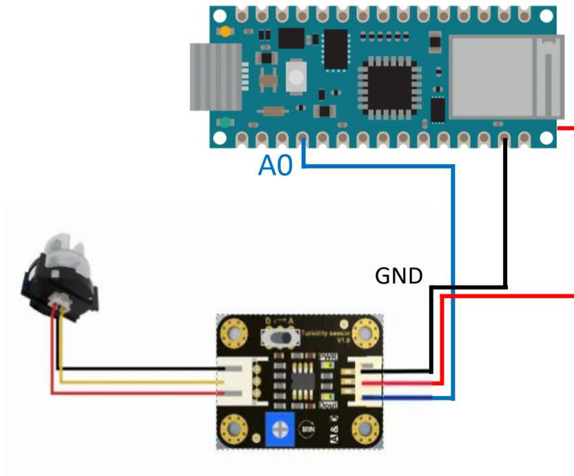
Connected to power supply of Arduino Nano 33 IoT that have been regulated
