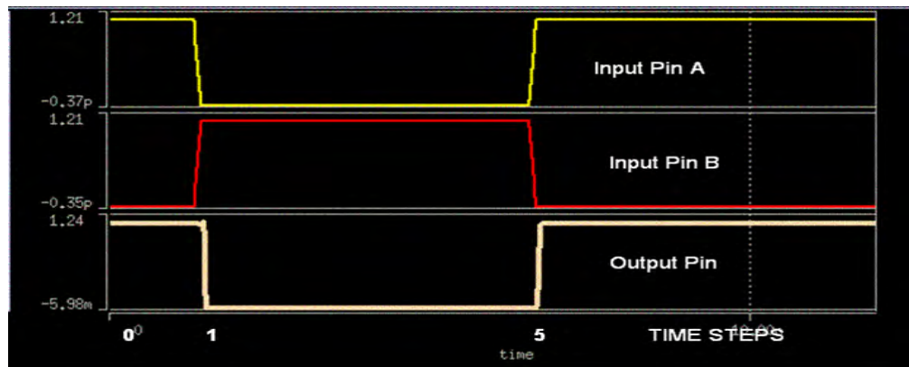
Figure 9-2 Signal profiles generated for a two-input combination cell.
