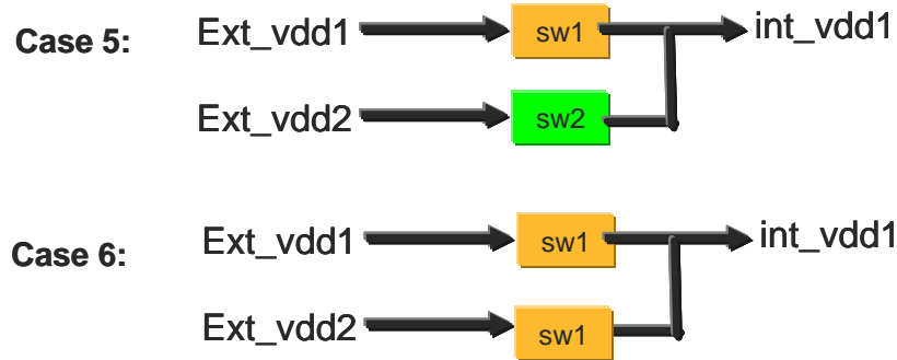
Figure 13-19 Unsupported switched RAM configurations
