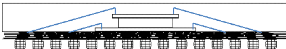
Figure 18-2 Configuration of SiP with two stacked dies, with spacer
