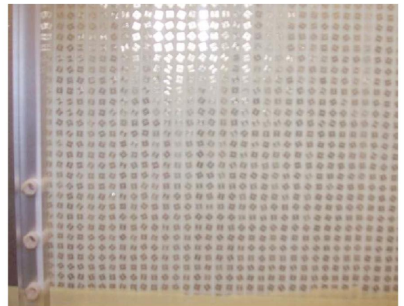
Fig. 2. Conformal metamaterial coating, FR4 dielectric sheet, 0.7 mm thick, on which a periodic, metallized patterns of mixed SRR shapes are printed.
