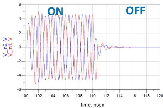
Before applied these signals at transistor gate, transistors are biased. I'm using HEMT as the switch transistor. It can only conduct drain current if the gate-source voltage  $> -4V$  as shown in the characteristic curve. That's the reason I bias the voltage for OFF-state below  $-4V$ , so no current will be conducted during this period.
