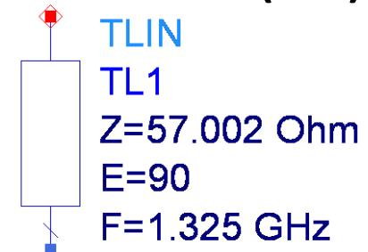
S-Parameter Simulation of Ideal Transmission Line based  $\lambda/4$  Impedance Transformer
