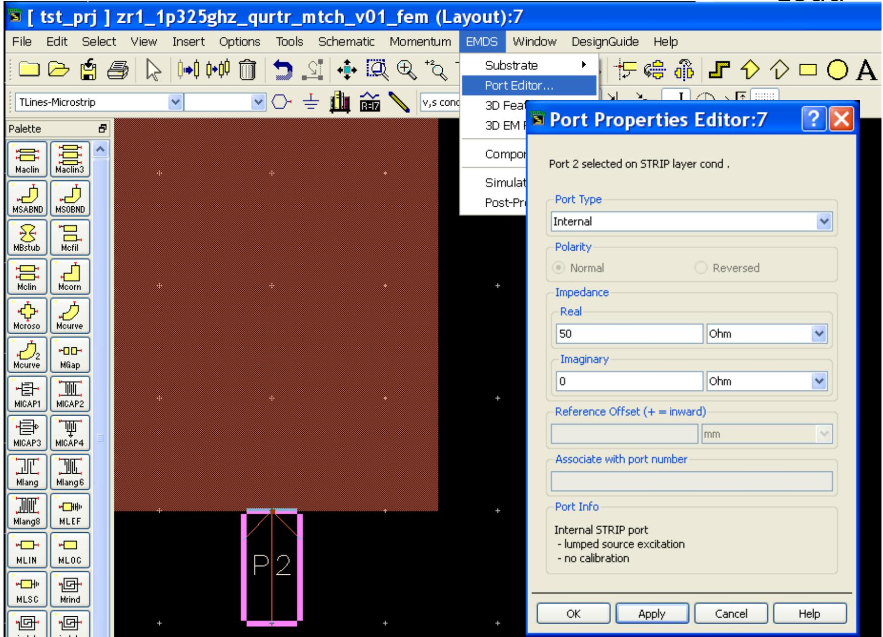
EMDS (FEM) based S-Parameters EM-circuit Co-Simulation of the  $\lambda/4$
