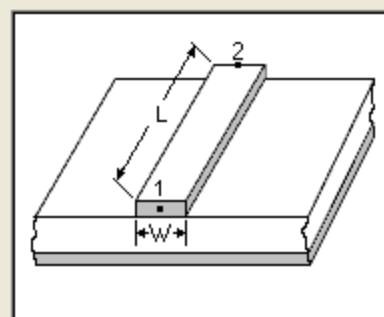
Layout Creation of the  $\lambda/4$  Microstrip Line Impedance Transformer
