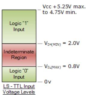
So for example, for the TTL 74LSxxx series of digital logic gates, the voltage ranges representing a logic level “1” and a logic level “o” are shown.
