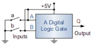
You may think that this would work fine as when switch “a” is open (off), the input is connected to Vcc (+5V) and when the switch is closed (on), the input is connected to ground as before, then inputs “A” or “B” always have a default state regardless of the position of the switch.
