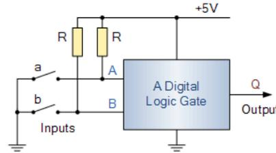
By using these two pull-up resistors, one for each input, when switch “A” or “B” is open (off), the input is effectively connected to the +5V supply rail via the pull-up resistor. The result is that as there is very little input current into the input of the logic gate, very little voltage is dropped across the pull-up resistor so nearly all the +5V supply voltage is applied to the input pin creating a HIGH, logic “1” condition.
