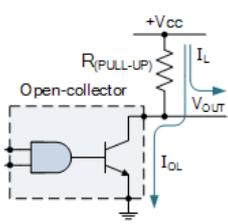
Logic gates, micro-controllers and other such digital circuits that have open-collector outputs, are incapable of pulling their outputs HIGH as there is no internal path to the supply voltage, ( $V_{CC}$ ). This condition means that their output is either grounded when LOW, or floating when HIGH, so an external pull-up resistor, ( $R_p$ ) needs to be connected from the open-collector terminal of the pull-down transistor to the  $V_{CC}$  supply.
