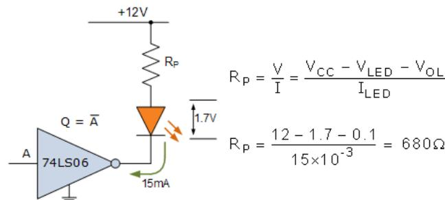
We can use open-collector drivers in a similar way to drive small electromechanical relays, lamps or dc motors as these devices typically require 5V or 12V or more, at a current of about 10 to 20 mA's to operate correctly.
