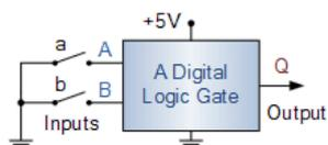
For example, consider the digital circuit on the left. The two switches, "a" and "b", represent the inputs to a generic logic gate. When switch "a" is closed (on), input "A" is connected to ground, (0V) or logic level "0" (low) and likewise, when switch "b" is closed (on), input "B" is also connected to ground, logic level "0" (low) and this is the correct condition we require.
