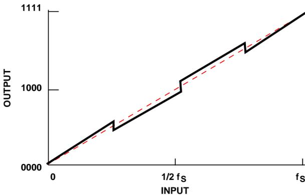
FIGURE 43B. SUCCESSIVE APPROXIMATION A/D CONVERTERS
