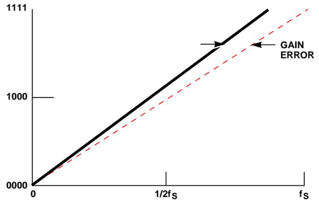
FIGURE 40B. GAIN ERRORS FOR AN A/D CONVERTER
