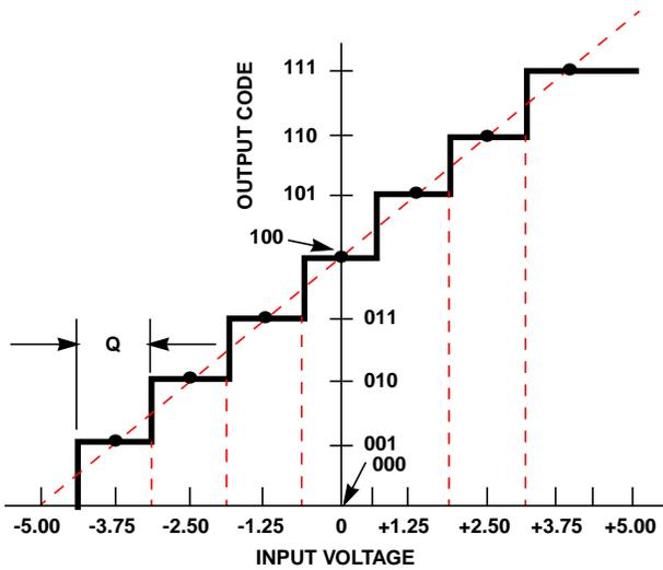
**FIGURE 9. TRANSFER FUNCTION FOR BIPOLAR 3-BIT A/D CONVERTER**
