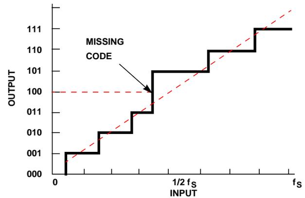
FIGURE 42B. A/D CONVERTER WITH MISSING CODE
