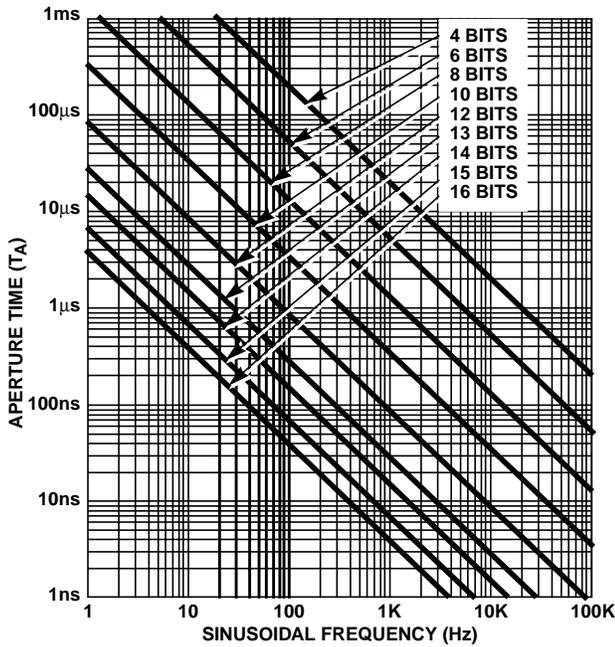
FIGURE 5. GRAPH FOR APERTURE ERROR FOR SINUSOIDAL SIGNALS
