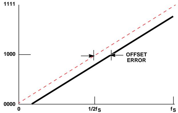
FIGURE 40A. OFFSET ERRORS FOR AN A/D CONVERTER
