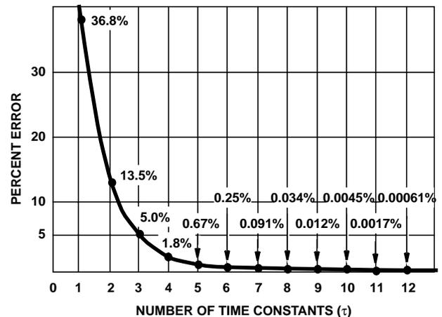
FIGURE 15. OUTPUT SETTLING ERROR AS A FUNCTION OF NUMBER OF TIME CONSTANTS
