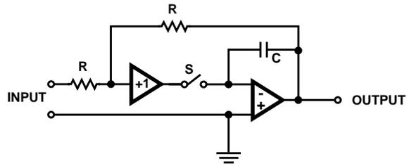
**FIGURE 38A. CLOSED LOOP SAMPLE-HOLD CIRCUIT**
