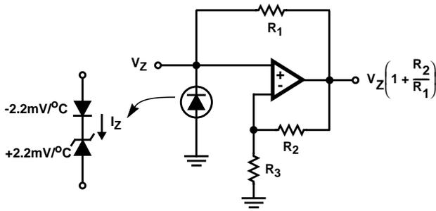
FIGURE 22. A PRECISION, BUFFERED VOLTAGE REFERENCE CIRCUIT
