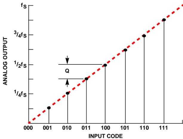
FIGURE 16. TRANSFER FUNCTION OF IDEAL 3-BIT D/A CONVERTER
