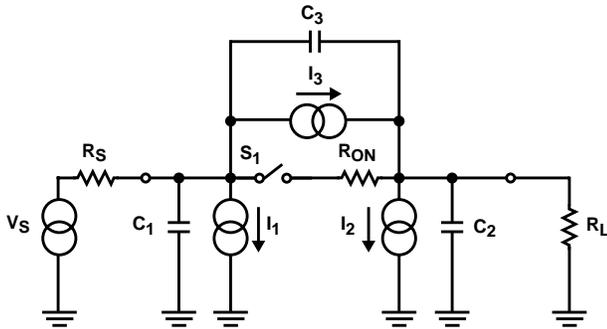
FIGURE 34. EQUIVALENT CIRCUIT OF ANALOG MULTIPLEXER SWITCH
