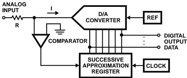
FIGURE 24. SUCCESSIVE APPROXIMATION A/D CONVERTER
