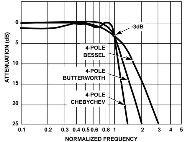
FIGURE 12. SOME PRACTICAL LOW PASS FILTER CHARACTERISTICS
