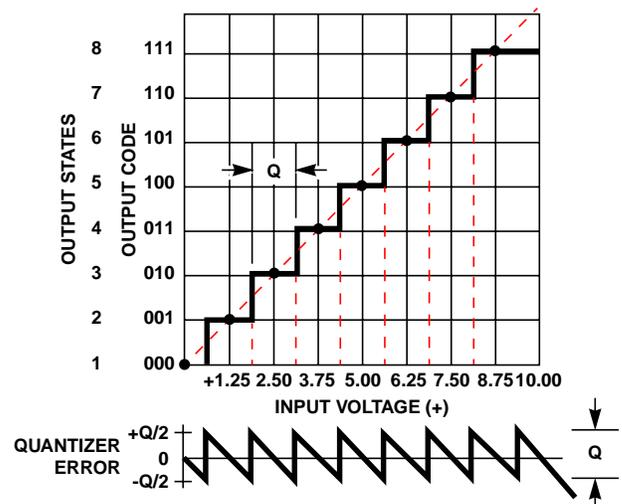
FIGURE 3. TRANSFER FUNCTION OF IDEAL 3-BIT QUANTIZER
