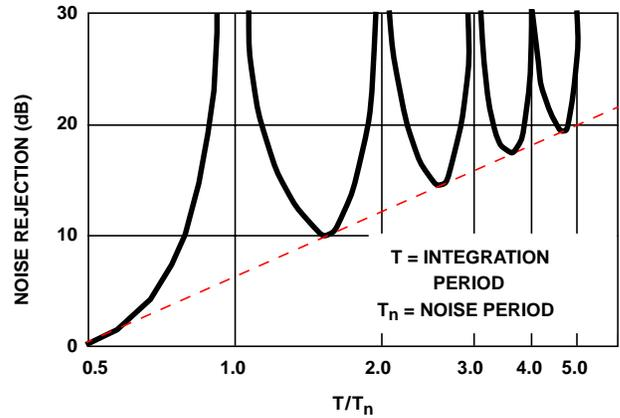
FIGURE 31. NOISE REJECTION FOR INTEGRATING TYPE A/D CONVERTERS
