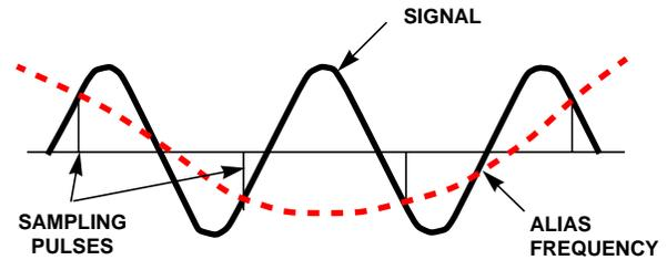
FIGURE 8. ALIAS FREQUENCY CAUSED BY INADEQUATE SAMPLING RATE
