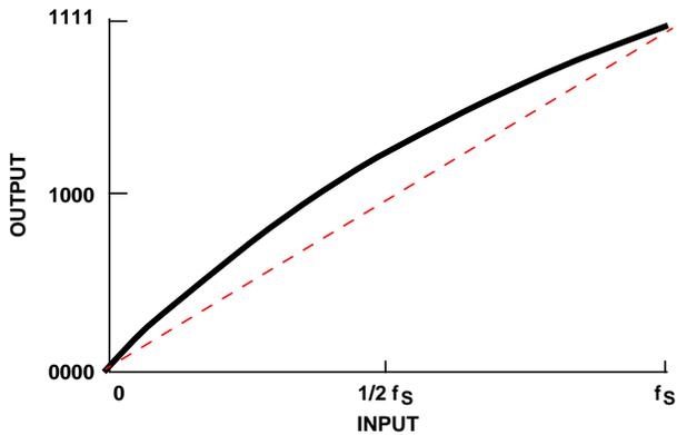
FIGURE 43A. LINEARITY CHARACTERISTICS OF INTEGRATING A/D CONVERTERS
