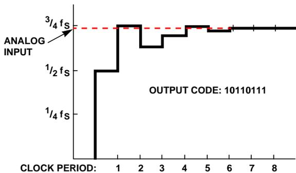
FIGURE 25. D/A OUTPUT FOR 8-BIT SUCCESSIVE APPROXIMATION CONVERSION
