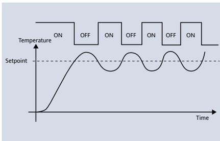
The amplitude and time period of the oscillation is a function of the thermal lag between the heating source and the temperature sensor.
