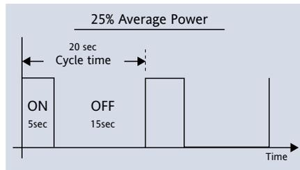
The cycle time must be short enough to allow the thermal mass of the load to smooth out the switching pulses. 20 seconds is typical. Systems with a small thermal mass will need shorter cycle times than can be provided with a relay. In these cases, a solid state relay is typically used with cycle times down to 0.2 seconds.
