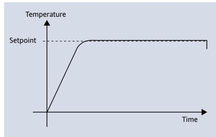
PID control is also referred to as "Three-term" control. The three terms are:
