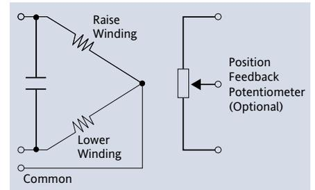
Eurotherm controllers provide a control algorithm specifically designed for use with motorised valves. This algorithm works equally well with or without a position feedback potentiometer.
