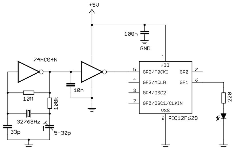
If the 32.768 kHz clock input is divided (prescaled) by 128, bit 7 of TMR0 will cycle at 1 Hz.
