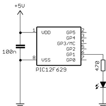
The LED is connected to the GP1 pin on a PIC12F629.
