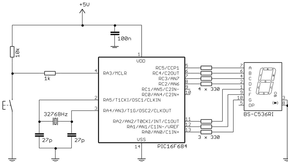
Timer1 is configured as before, driven by the 32.768 kHz crystal:
