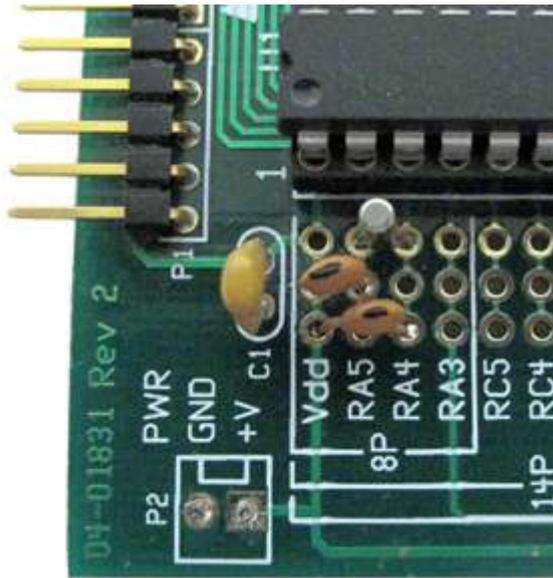
Note that the capacitors in the picture are **not** connected as per the circuit diagram! For convenience (the layout is a lot simpler), they are connected between the crystal and VDD (+5V), not ground. This works because capacitors block DC; as far as the crystal is concerned, its load capacitors are grounded, because the capacitors block the DC component of the 5 V supply.
