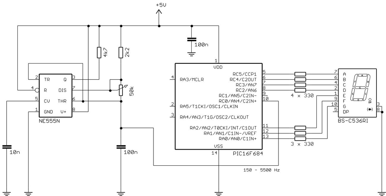
The code is very similar to that in the previous example; the only differences being that we need to configure the comparator, select the comparator gate control mode, and poll the comparator output instead of the digital input.
