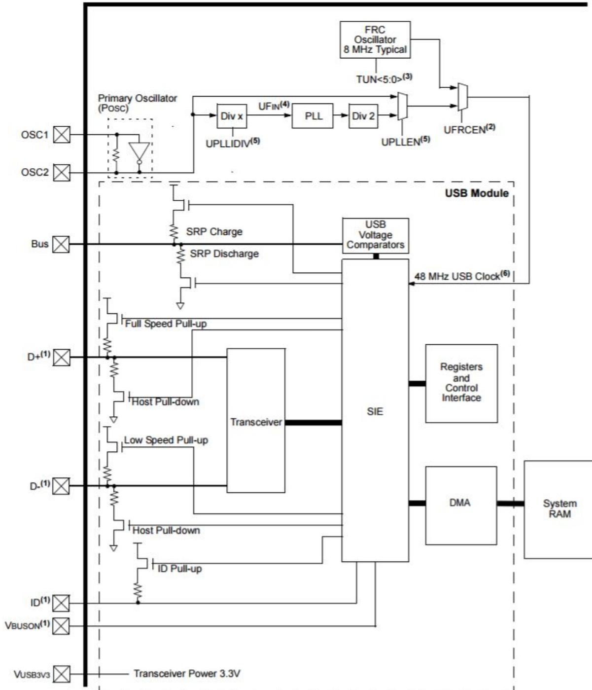
**Figure 9:** USB Module Hardware
