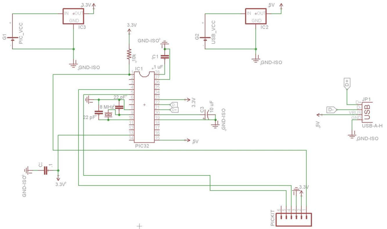
**Figure 12:** Minimal USB Circuit for Stand-alone PIC32 Using PICKIT 3
