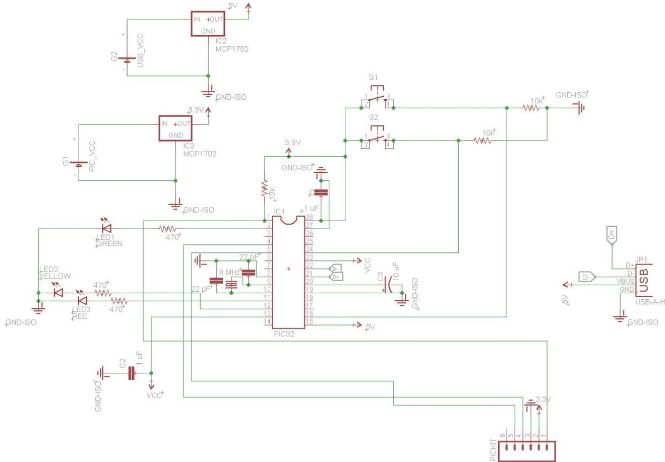
**Figure 11: Functional Circuit for Interfacing Standalone PIC32 with MSD**
