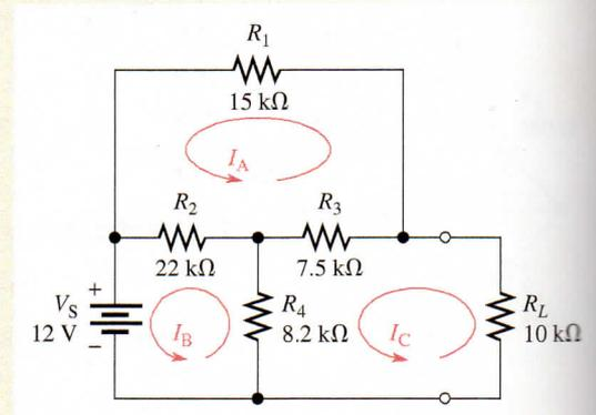
**Solution** Assign three counterclockwise loop currents ( $I_A$ ,  $I_B$ , and  $I_C$ ) as shown in Figure 9-14. Write the loop equations, but drop the k prefix from the resistances. Current will be in mA.
