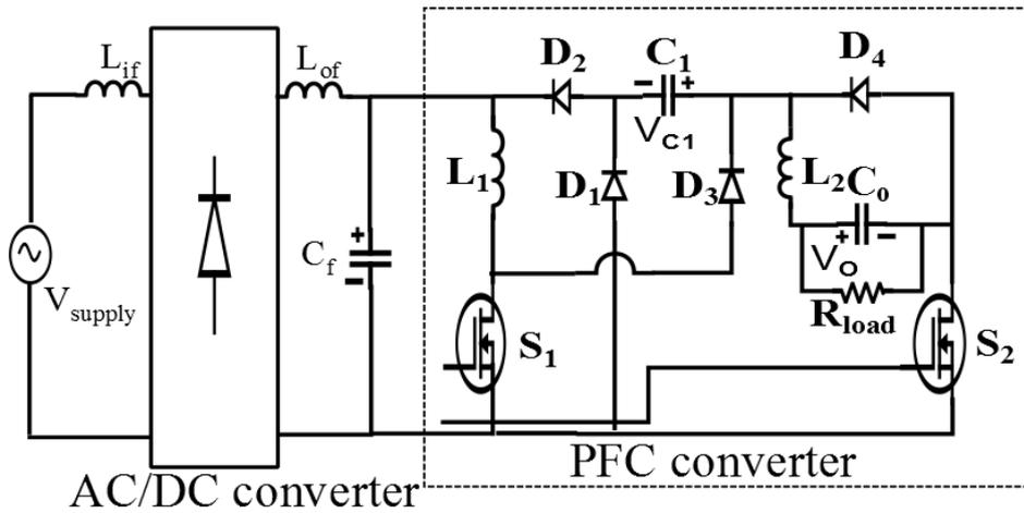
The input buck-boost stage is formed by  $L_1, S_1, D_2, D_3, C_1 \dots$ . The output buck stage is formed by  $C_1, L_2, C_o, S_2, D_1, D_4$  with  $C_1$  as intermediate energy storing capacitor. Both stages operate in DCM..I have shown the complete operation of the PFC in four modes
