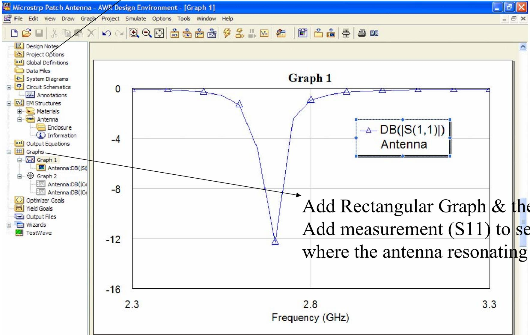
Add Rectangular Graph & then Add measurement (S11) to see where the antenna resonating
