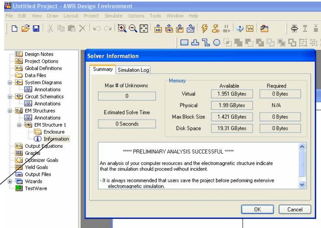
Check memory requirement and recommended cache. They should be less than your physical memory and Max cache size, respectively.
