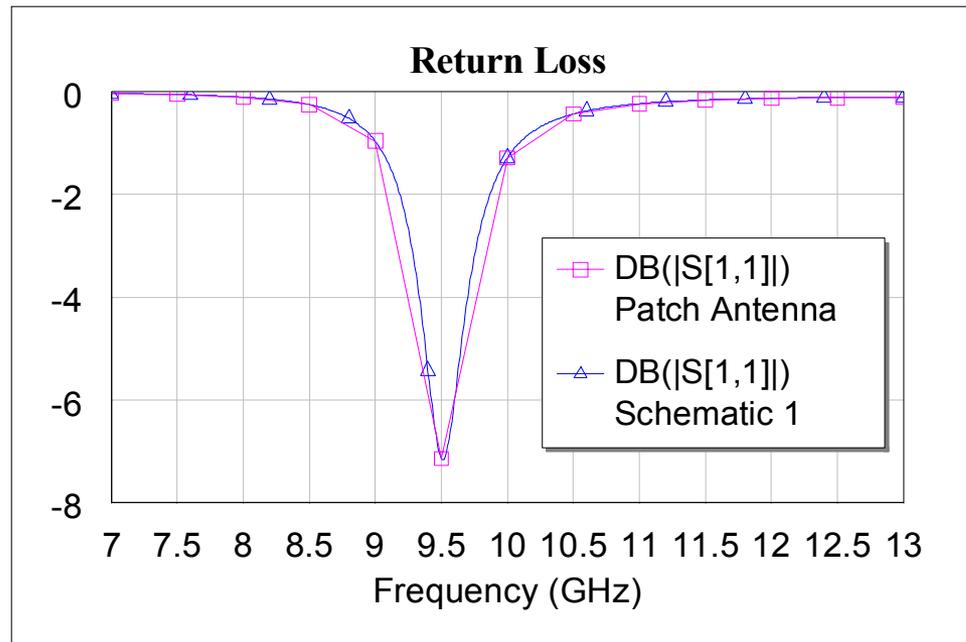
Add a few more frequency point to EM Structure frequency range after you know the location of the resonant frequency.
