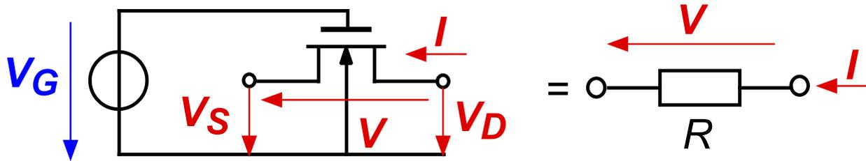
In linear mode:  $I = \beta(V_D - V_S)[V_G - V_{T0} - \frac{n}{2}(V_D + V_S)]$
