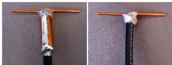
Fig. 9 Dipole with and without Sleeve Balun
