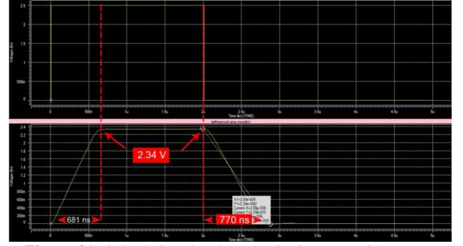
Figure 21. Calculating the slew rate in Op-amp with current buffer and miller capacitor
