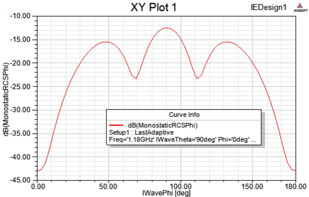
This is the HH monostatic RCS pattern for the standard ogive at 1.18GHz.
