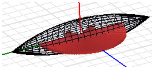
This will solve for the response due to incident planes waves that are incident in the  $\theta=90^\circ$  and for  $\phi=0$  to  $180^\circ$  for 61 values. The polarization is  $\phi$  directed so we will be solving for the HH monostatic RCS.
