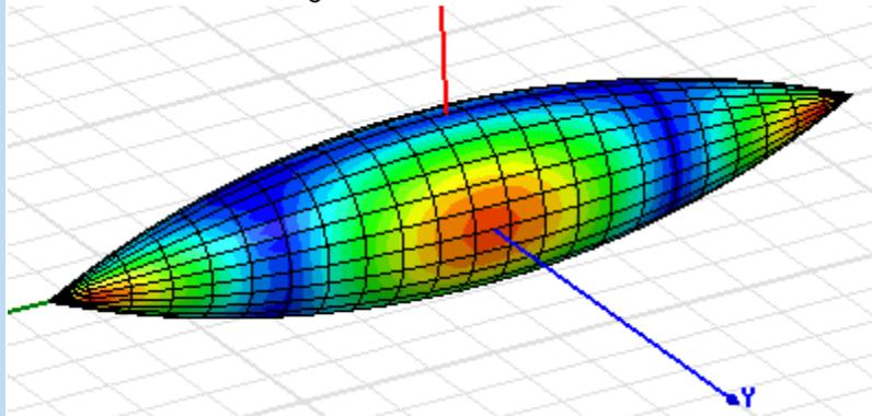
We will look at the scattering from a conducting ogive with a length of 10" and a half angle of  $22.6^\circ = 0.3948$  radians. The ogive lies with its axis along the x axis. The equation that defines this model is:
