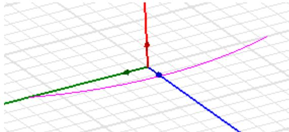
Look in the **History** tree under Lines and Equation Curve1 and double-click on CreateEquationCurve. This lets you view the command **Properties** window which includes the setup shown, with the Value column expanded for complete viewing.
