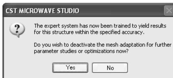
This dialog box informs you that the desired accuracy limit (2% by default) could be met by the adaptive mesh refinement. Because the expert system's settings have now been
