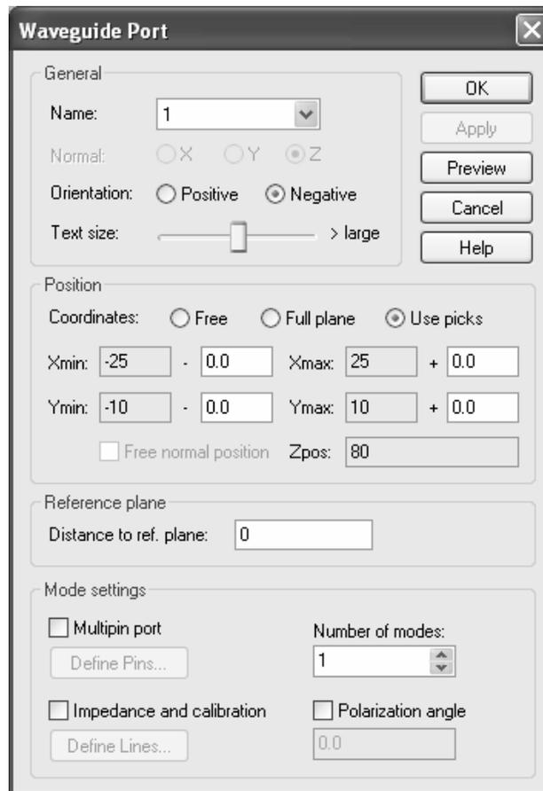
In this case, you can simply accept the default settings and press **OK** to create the port. The next step is the definition of ports 2, 3 and 4.
