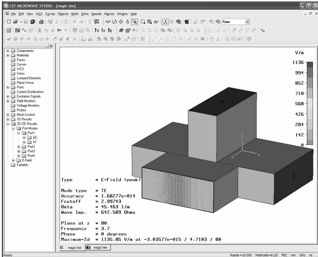
Because we have selected the main entry, a 3D vector plot is shown. Selecting either of the subentries will produce a scalar plot. The plot also shows some important properties of the mode such as mode type, cut-off frequency and propagation constant. The port modes at the other ports can be visualized in the same manner.
