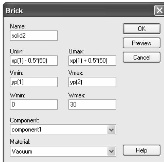
Some of the coordinate fields now contain mathematical expressions because some of the points were entered using the pick tools. Here, the functions  $xp(1)$ ,  $yp(1)$  represent the point coordinates of the first picked point (the midpoint of the first brick's lower edge). Analogously, the functions  $xp(2)$  and  $yp(2)$  correspond to the upper edge's midpoint.
