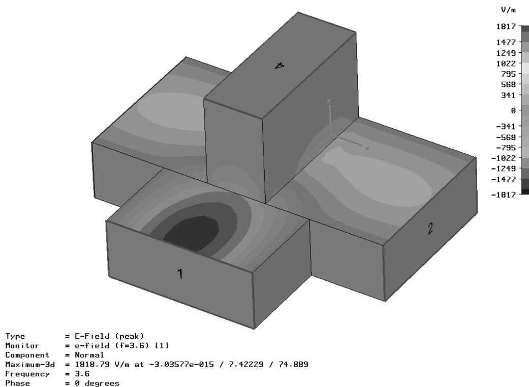
You can display an animation of the fields by checking the *Animate Fields* option in the context menu (right mouse click in the plot window). The appearance of the plot can be changed in the plot properties dialog box, that can be opened by selecting *Results* ⇨ *Plot Properties* from the main menu or *Plot Properties* from the context menu. Alternatively, you can double-click on the plot to open this dialog box.
