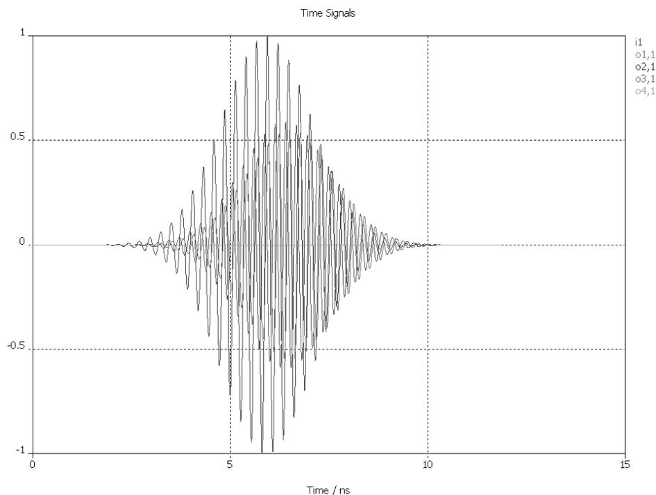
This plot shows the incident and reflected or transmitted wave amplitudes at the ports versus time. The incident wave amplitude is called  $i1$ , the reflected wave amplitude is  $o1,1$  and the transmitted wave amplitudes are  $o2,1$ ,  $o3,1$  and  $o4,1$ . You can see that the transmitted wave amplitudes  $o2,1$  and  $o3,1$  are delayed and distorted (note that  $o2,1$  and  $o3,1$  are identical, so do not be concerned if you only see one curve).
