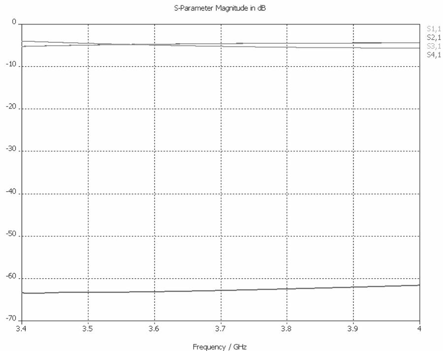
Similar to the case of transient solver, an extremely small transmission to port 4 (S4,1) is observed here. In addition, you can conclude that the other S-parameters have at least the same order of magnitude as the S-parameters computed with the transient solver.
