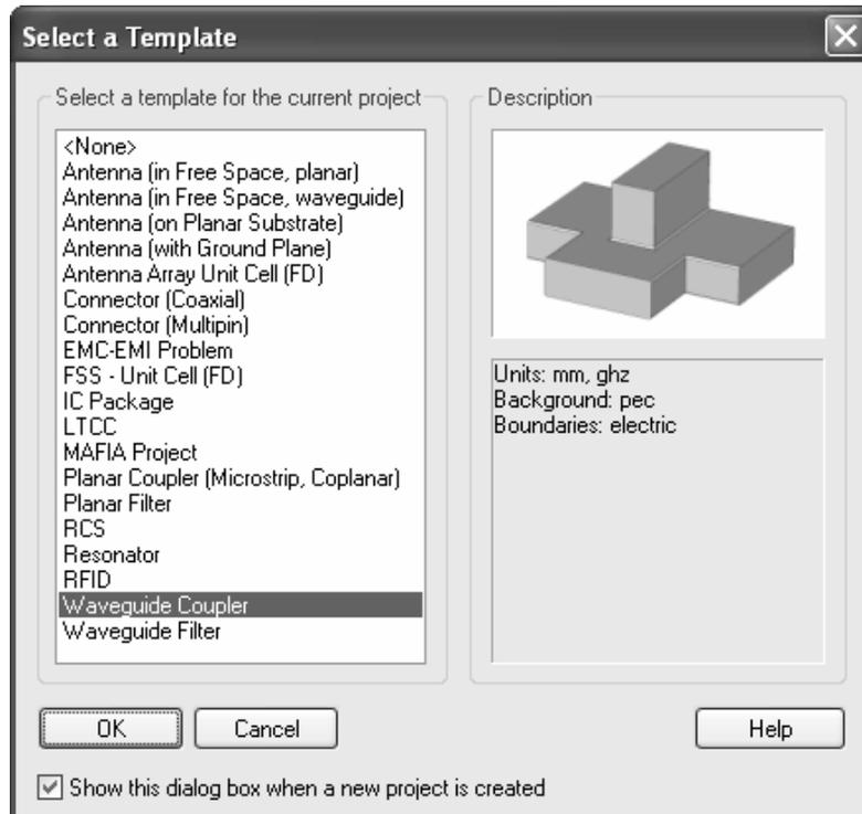
This template automatically sets the units to mm and GHz, the background material to PEC (which is the default) and all boundaries to be perfect electrical conductors.
