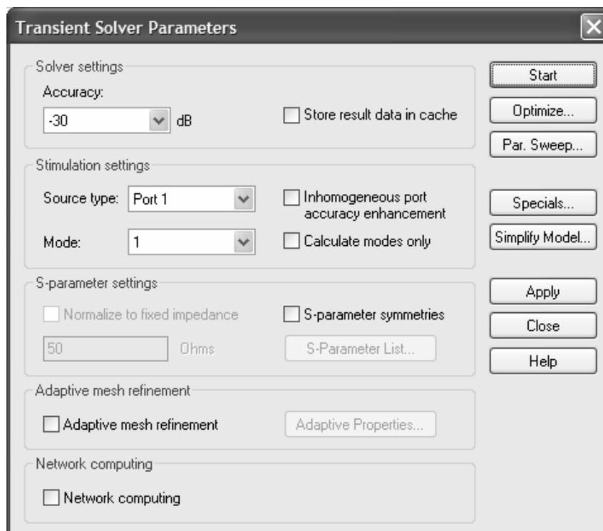
You should now specify whether the full S-matrix should be calculated or if a subset of this matrix is sufficient. For the Magic Tee device we are interested in the input reflection at port 1 and in the transmission from port 1 to the other three ports (2, 3 and 4).
