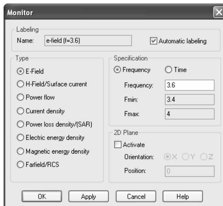
In this example, you should define an electric field monitor (*Type = E-Field*) at a *Frequency* of 3.6 GHz before pressing the *OK* button to store the settings. The green box indicates the volume in which the fields will be recorded.
