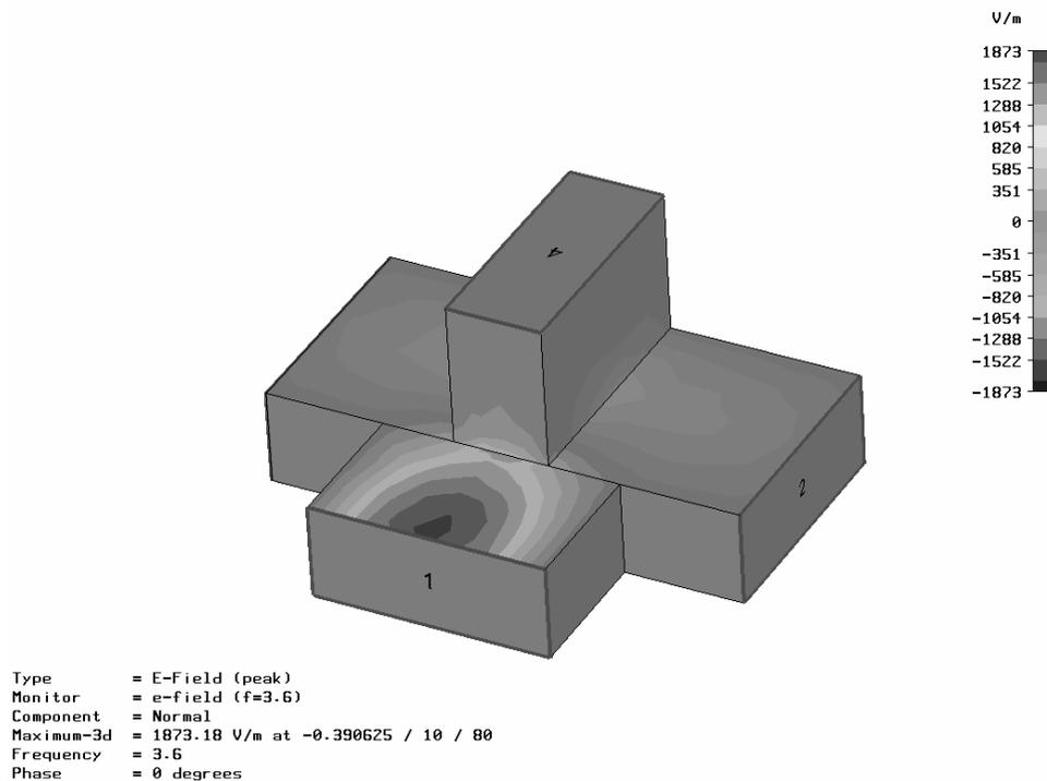
Here, you can observe the effect of the coarse tetrahedral mesh on the computed field: the contours of the computed field distribution are slightly irregular. The next section describes how to influence the mesh refinement and improve the quality of the computed field distribution.
