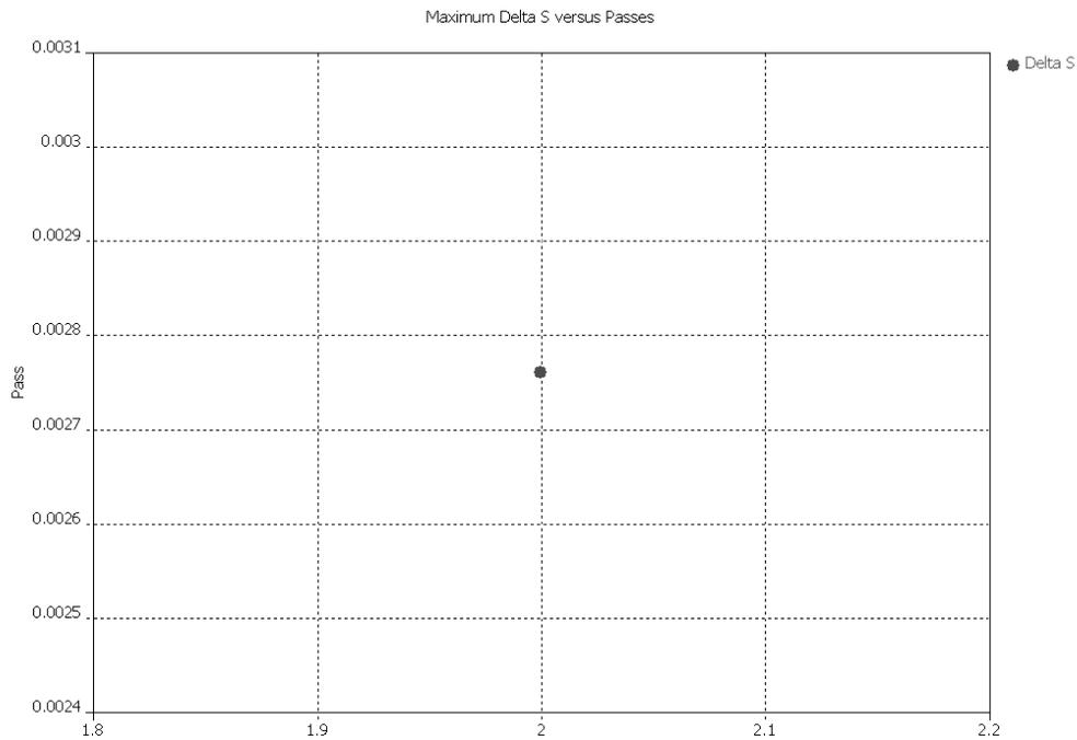
As you can see, the maximum deviation of the S-parameters is below 0.5%, indicating that the expert system based meshing would have been fine for this example even without running the mesh adaptation procedure.
