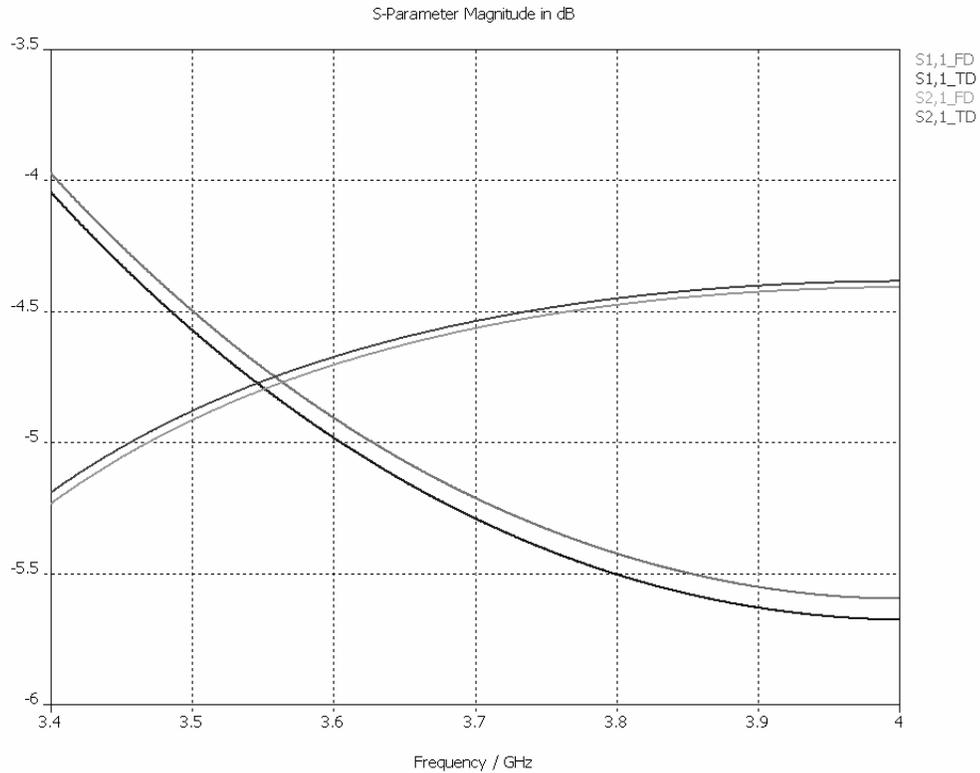
As you can see, the results agree very well. For this specific structure, the transient solver does provide more accurate results by default. The accuracy of the frequency domain simulation can be increased by lowering the accuracy limit for the adaptive mesh refinement.
