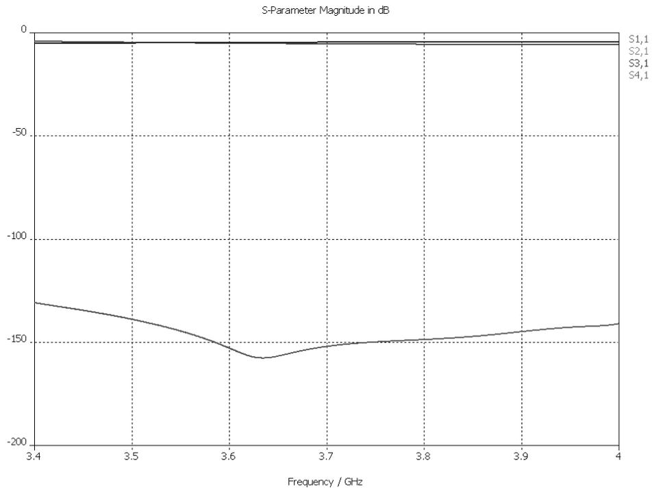
As expected, the transmission to port 4 ( $S_{4,1}$ ) is extremely small (-150 dB is close to the solver's noise floor). It is obvious that this simple device is very poorly matched so that the transmission to ports 2 and 3 is of the same order of magnitude as the input reflection at port 1.
