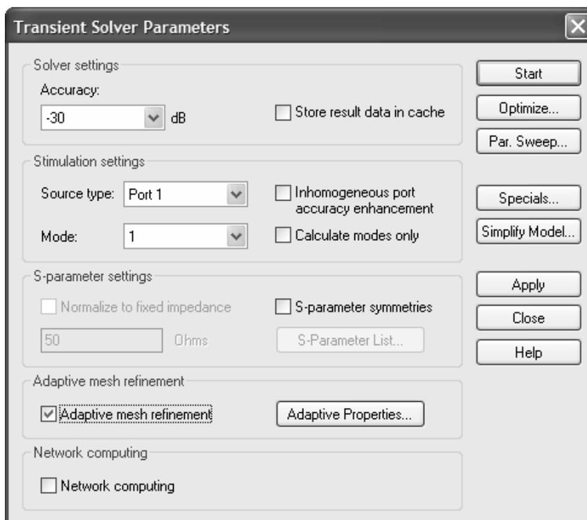
After activating the adaptive mesh refinement tool, you should now start the solver again by pressing the *Start* button. After a couple of minutes (during which the solver is running through mesh adaptation passes), the following dialog box will appear:
