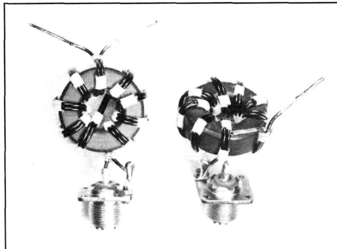
Photo J— Two medium-power versions of the bifilar toroidal (Guanella/current) 1:1 balun capable of handling the full legal limit of amateur radio power when the VSWR is less than 2:1. The balun on the left has the cross-over.
