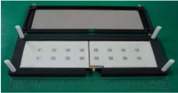
(b) Disassembled antenna structure
