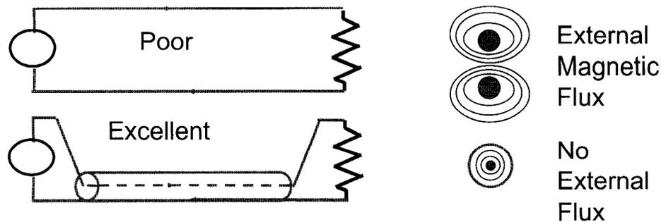
**If the return current can completely enclose the signal current, excellent magnetic field containment will result. Any techniques that will reduce self-inductance will also reduce or eliminate magnetic fields.**
