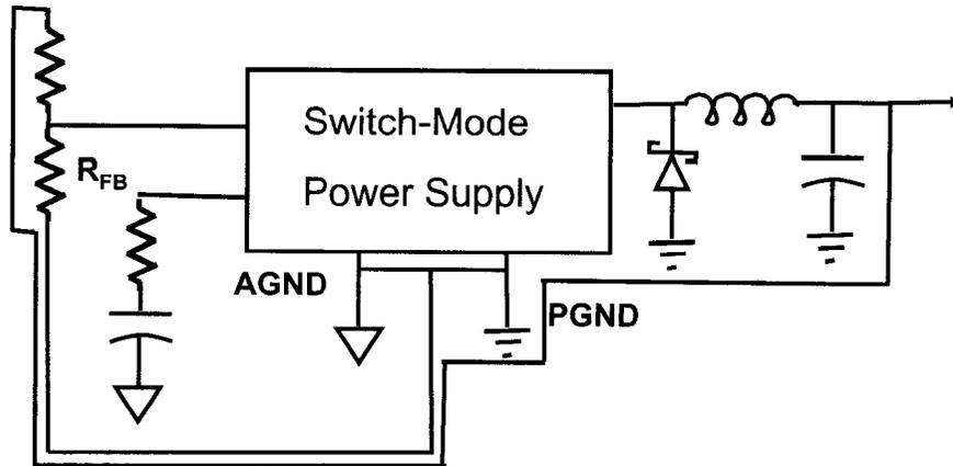
Connect AGND and PGND together at the chip  $R_{FB}$ . You must have a signal-return path to the AGND/PGND-junction point. Minimize the loop area for AGND and PGND circuits. Feedback resistors should be physically close to the feedback pin. Power and signal-return (ground) connections should be run close together to minimize loop area.
