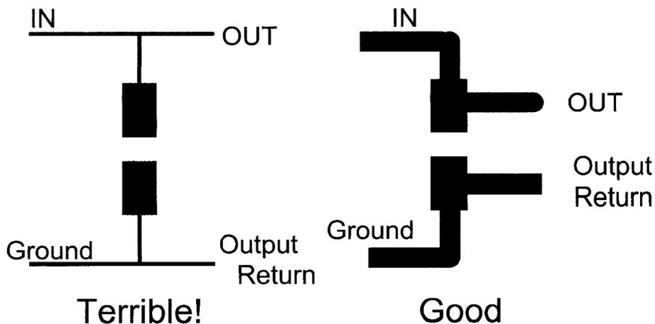
Take a look at the two layouts above. An output capacitor is intended to be connected to the surface-mount pads in each case. The design on the left will not do a very good job of reducing ripple and spikes due to the high inductance connections to it. The straight-through connection paths from the input to the output is likely a lower impedance path than the path through the capacitor.
