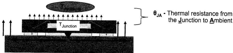
At each interface from the junction to the ambient air there is an associated thermal resistance
