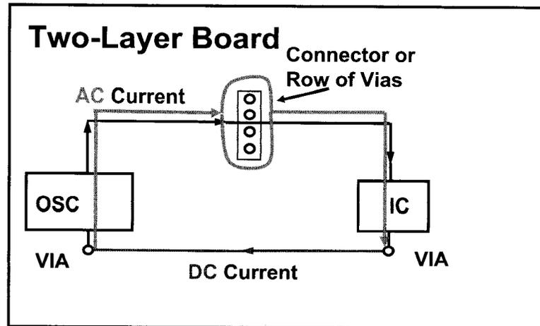
Row of vias opens up ground plane between pins and causes AC-return current to flow around gap in plane. The gap will radiate at whatever frequency is  $\frac{1}{4} \lambda = \text{gap length!}$
