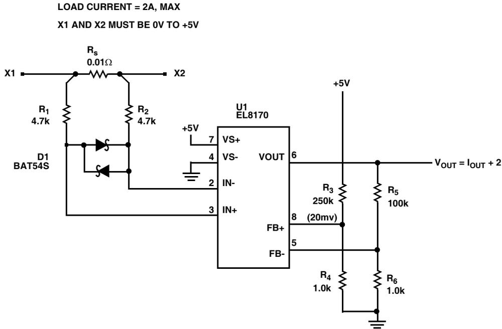
FIGURE 53. CURRENT MONITORED WITH LOW VALUE RESISTOR
