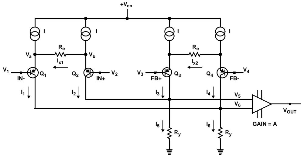
FIGURE 9. SIMPLIFIED SCHEMATIC
