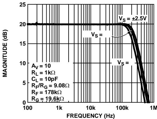
FIGURE 33. EL8171 FREQUENCY RESPONSE vs SUPPLY VOLTAGE
