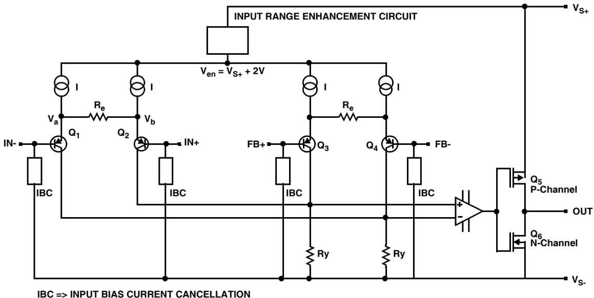
FIGURE 11. SIMPLIFIED SCHEMATIC
