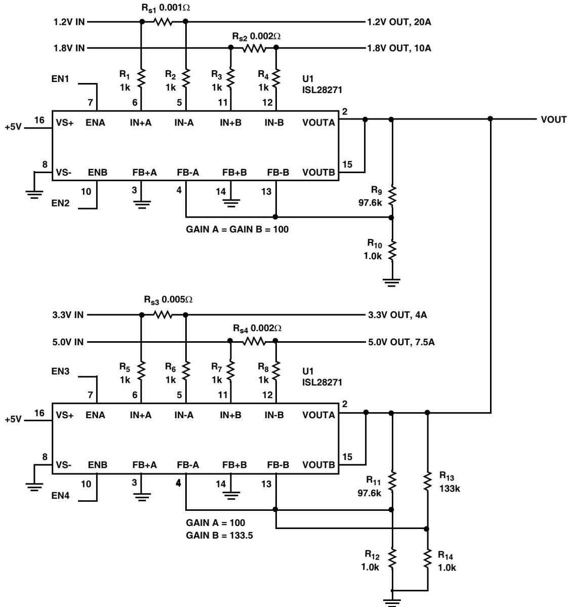
FIGURE 52. MEASUREMENT OF POSITIVE AND NEGATIVE CURRENT FLOW
