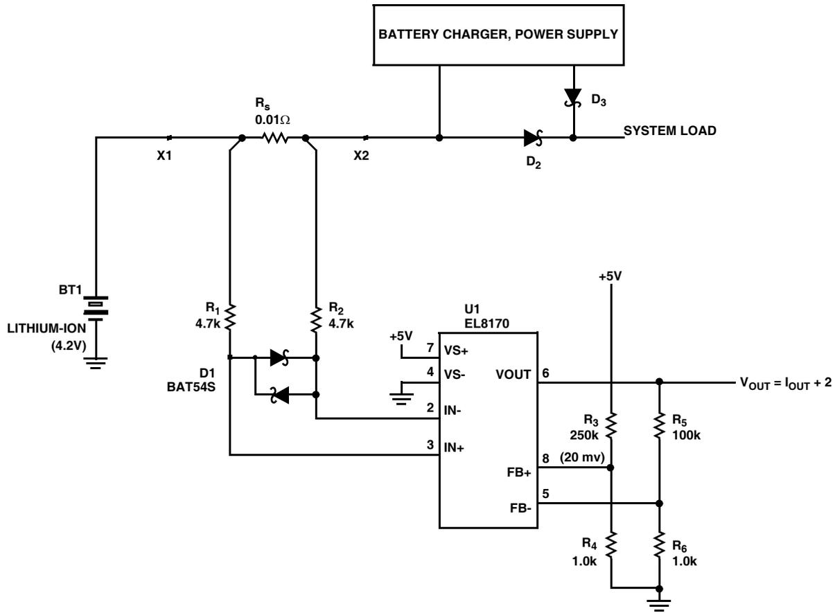
FIGURE 54. EL8170 SETUP AS A BATTERY CHARGER
