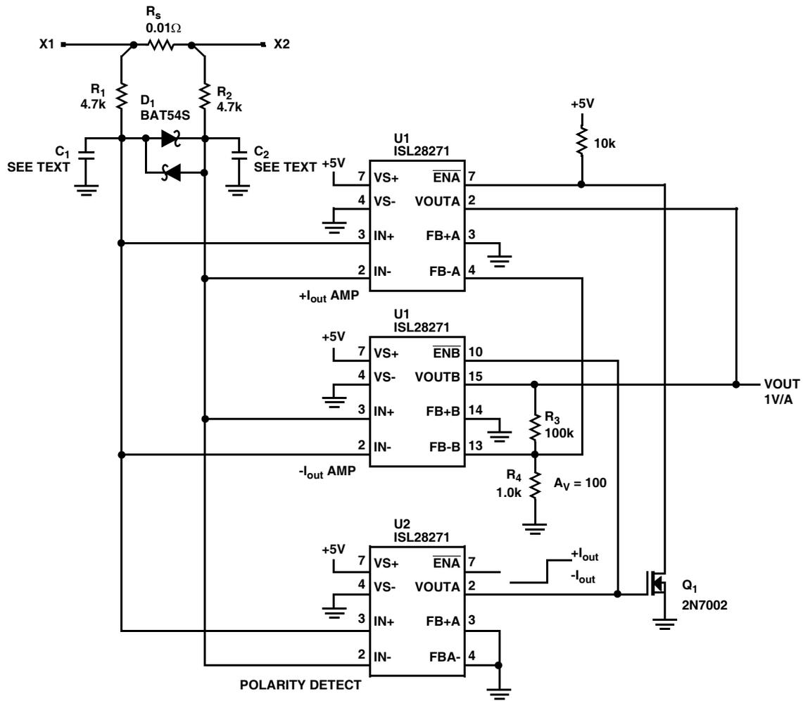
FIGURE 55. MEASUREMENT OF POSITIVE AND NEGATIVE CURRENT FLOW
