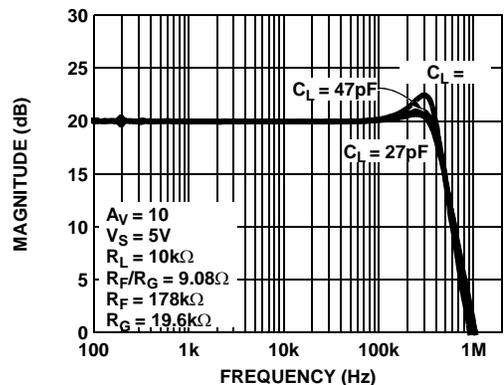
FIGURE 34. EL8171, EL8172 FREQUENCY RESPONSE vs  $C_{LOAD}$
