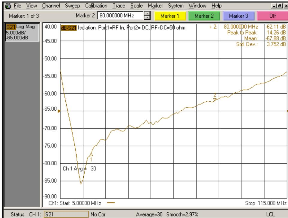
Figure 12 – Single Bias-T - Isolation between RF and DC Port *with* Capacitive Shunt (0.1  $\mu$ F).
