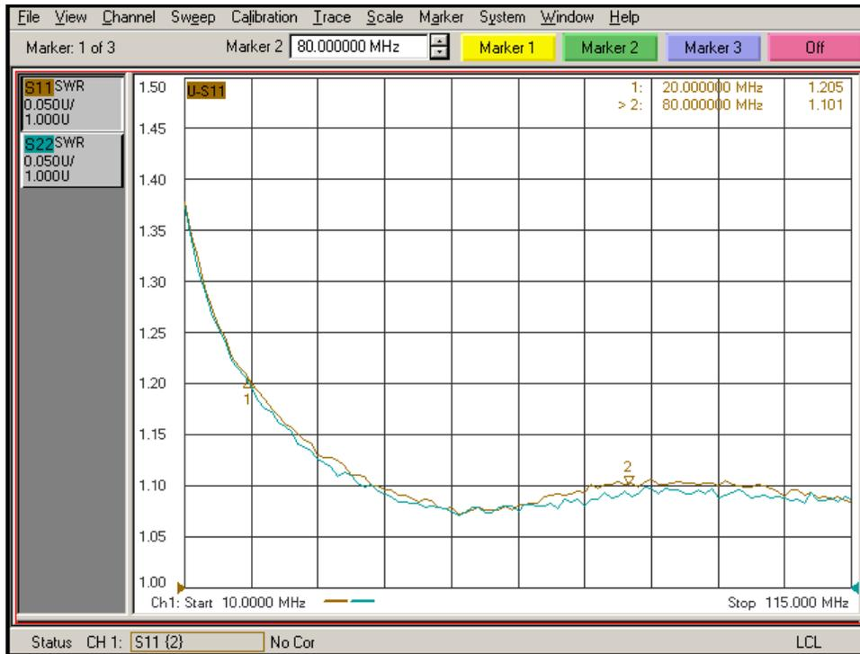
Figure 10 – SWR (S11 and S22) into Two Cascaded Bias-Ts Delivering 240 mA
