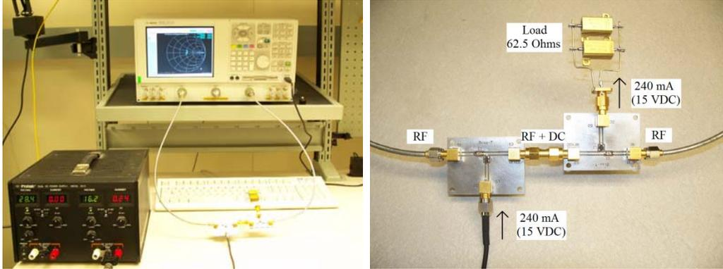
Figure 3 – Characterization of the Bias-T Operating under Load
