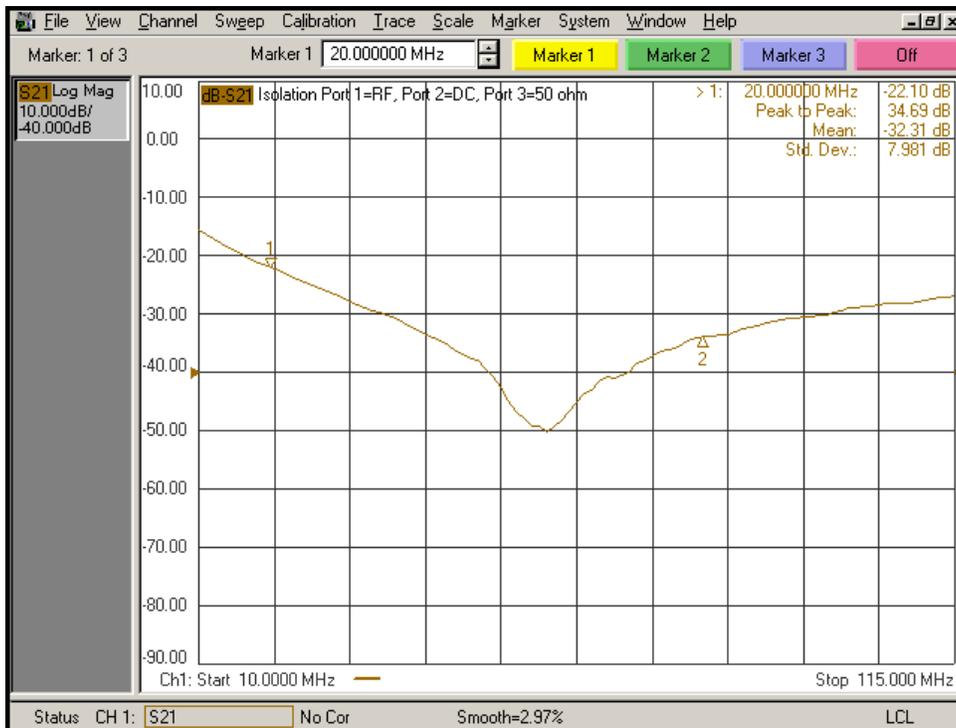
Figure 11 – Single Bias-T Isolation between RF and DC Port *without* Capacitive Shunt. RF+DC Port 50Ω Terminated
