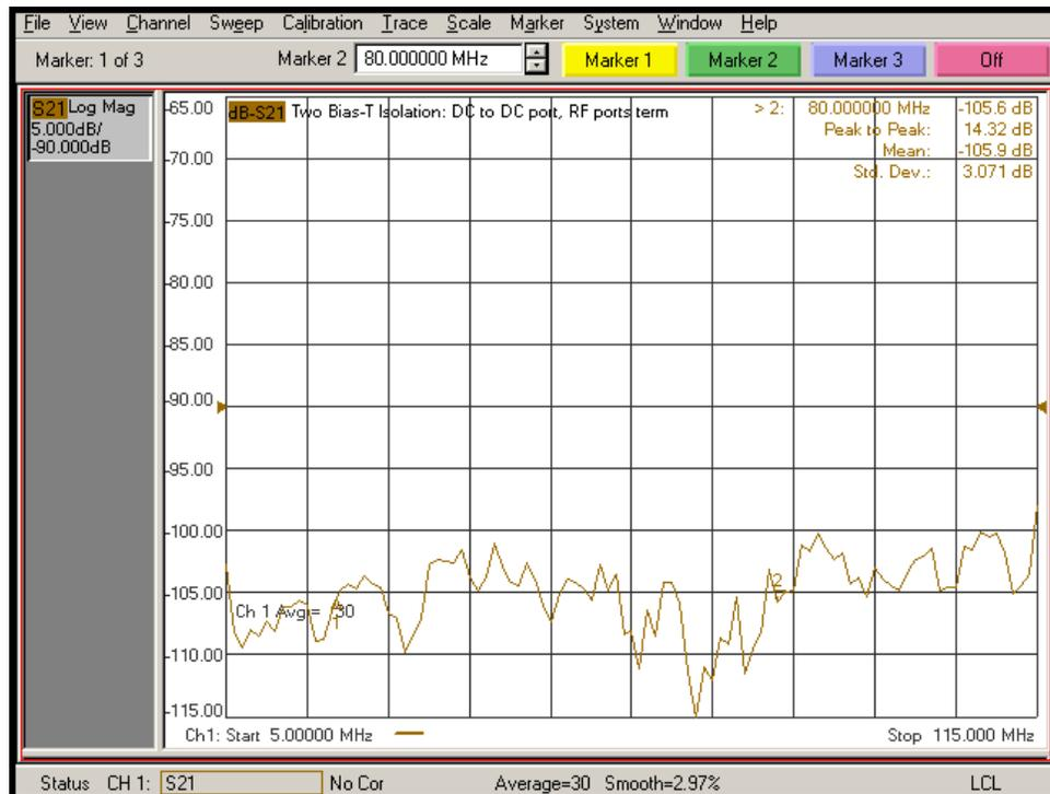
Figure 13 – Two Bias-Ts - Isolation between RF and RF Port *with* Capacitive Shunts (0.1  $\mu$ F).
