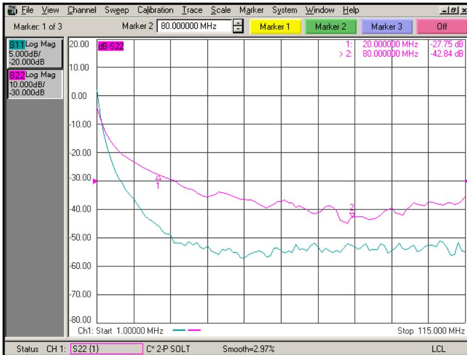
Figure 5 – Return Loss (S11 and S22) into a Single Bias-T with DC Port Shorted
