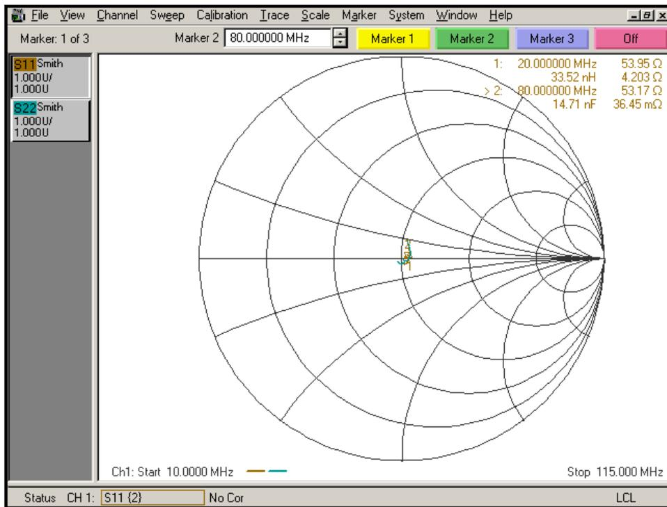
Figure 6 – Return Loss (S11 and S22) into a Single Bias-T with DC Port Shorted (Smith)
