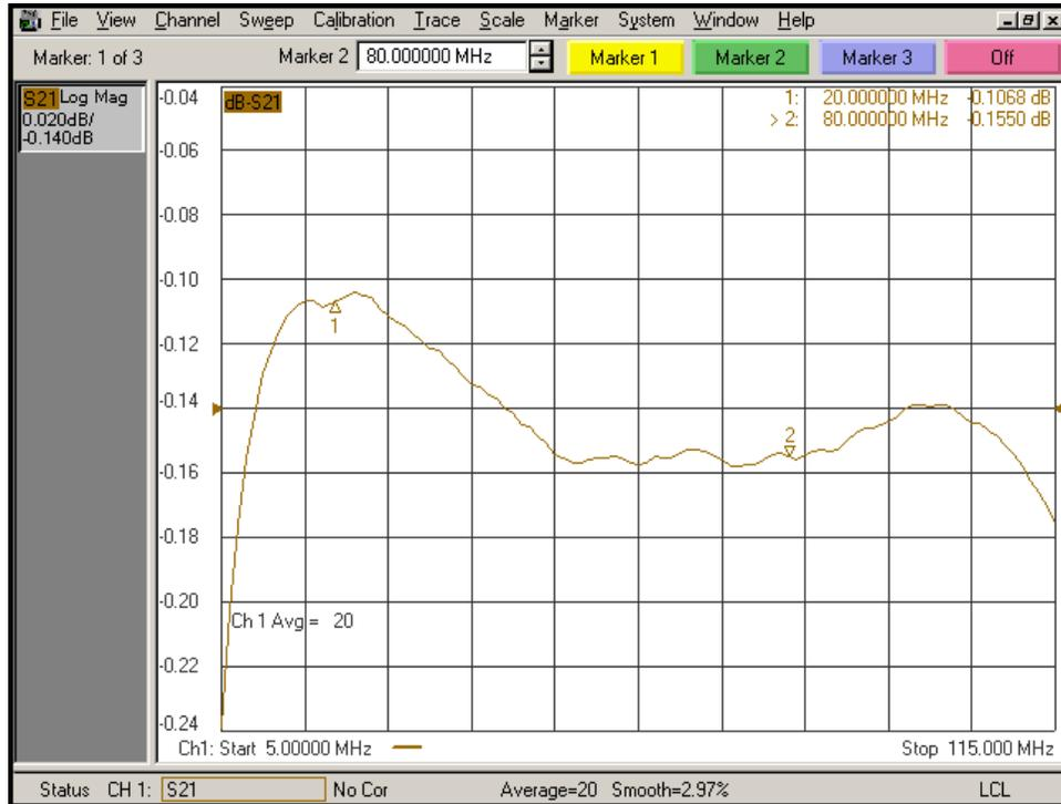
Figure 4 – Insertion Loss (S21) through a Single Bias-T with DC Port Shorted
