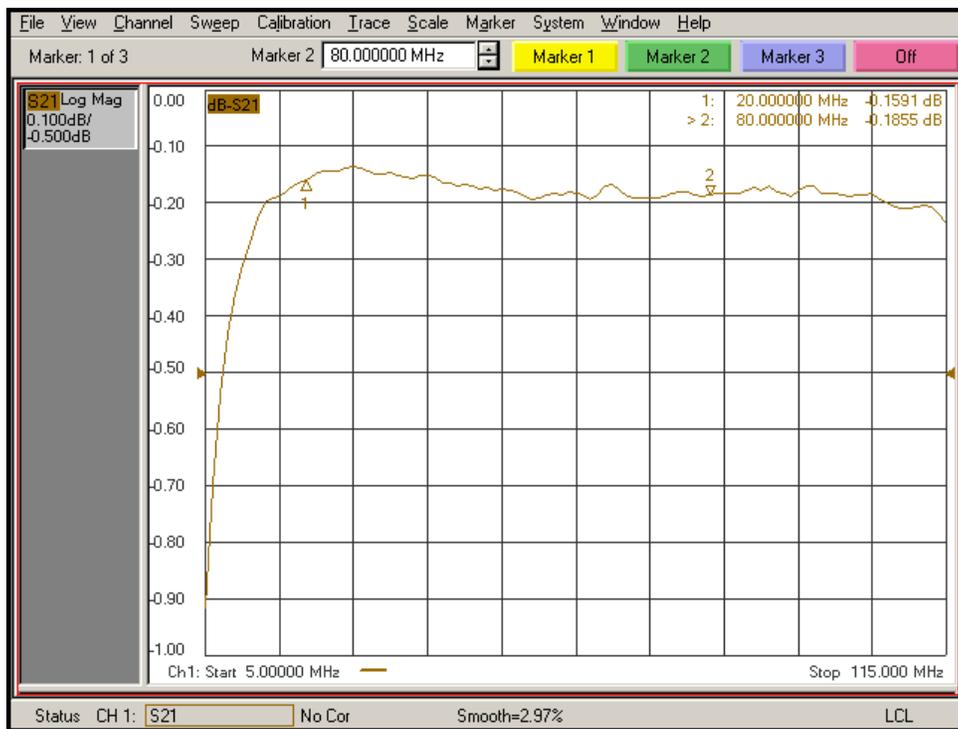
Figure 7 – Insertion Loss through Two Bias-T Supplying 240 mA to a Resistive Load
