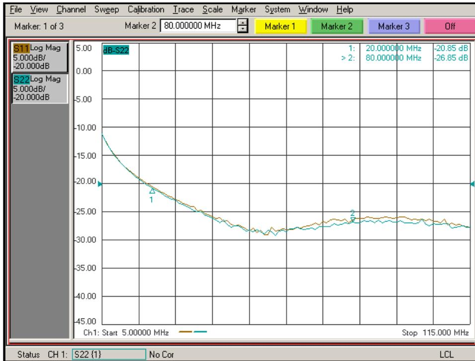
Figure 8 – Return Loss (S11 and S22) into Two Cascaded Bias-Ts Delivering 240 mA
