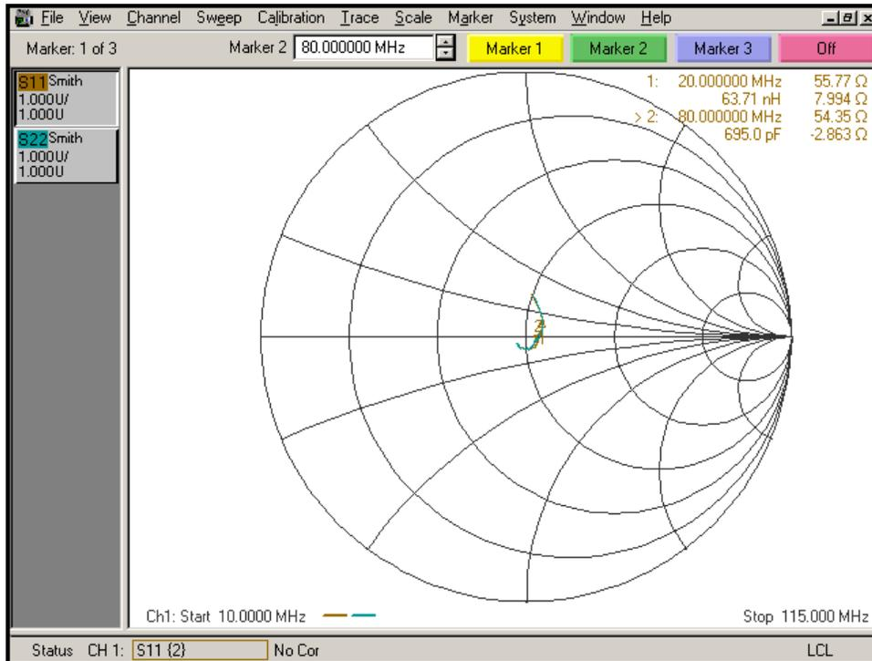
Figure 9 – Return Loss (S11 and S22) into Two Cascaded Bias-Ts Delivering 240 mA (Smith)
