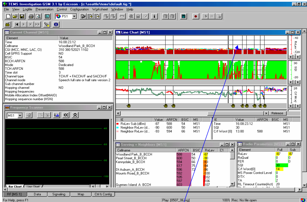
Figure 23– Lack of Dominant Server: Signals of more than one cell can be reaching a spot with low level causing ping pong handovers. This might happen because the MS is located on the cell borders and there is no any best server to keep the call.
