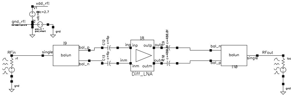
LNA design is a compromise among power, noise, linearity, gain, stability, input and output matching, and dynamic range. They are characterized by the design specifications in Table in page 4.
