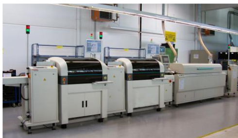
Building of production lines is simple due to standardized transport systems and interfaces.
