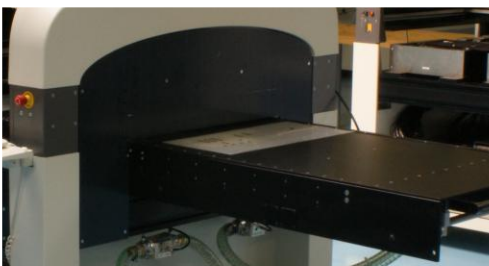
The vacuum table holds flex-boards securely. Different configurations are available with or without shuttle system.
