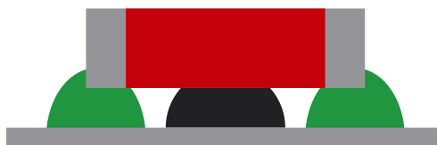
LED assembly onto flexible substrate using conductive epoxy (green) and additional glue (black) providing mechanical strength.
