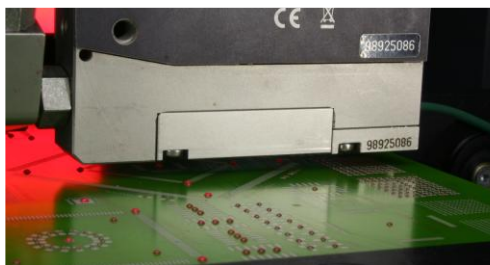
High speed dispensing of glue using a Jet dispensing valve.
