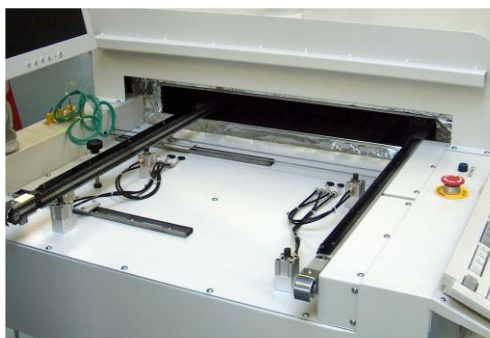
Special oven for soldering of LEDs onto polyester foils, a customer specific adaptation of the reflow oven RO300FC.
