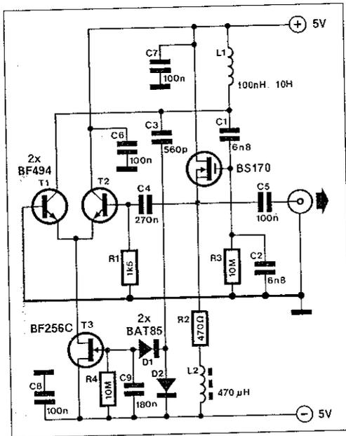
This compact LC oscillator offers a frequency range of about 1 kHz to almost 9 MHz and a low-distortion sine wave output.
