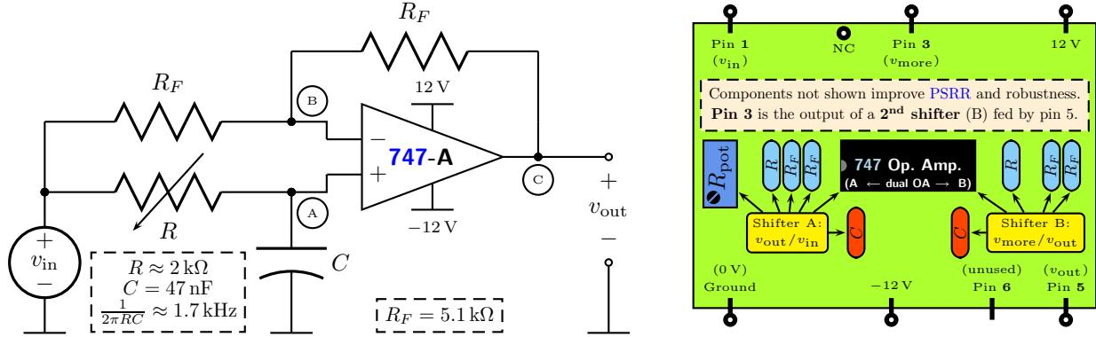
Intuitively, the phase shifter uses a first-order low-pass filter to create a phase shift and negative feedback to compensate for non-unity gain. The result is an all-pass filter that has input-to-output quadrature (i.e., quarter-wavelength, or \$90^\circ\$, phase shift) at \$\omega = 1/(RC)\$ (i.e., \$f = 1/(2\pi RC)\$).
