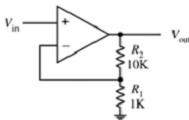
$$Gain = \frac{V_o}{V_i} = 1 + \frac{R_2}{R_1}$$
