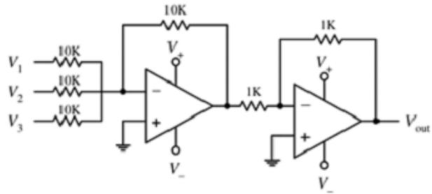
$$V_o = V_1 + V_2 + V_3$$
