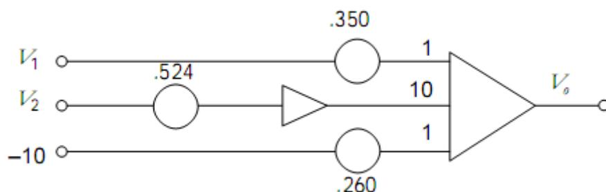
Note the inversion operation of all inputs that is because the summer inverts the output as we introduced before and the inverter must have a unity gain.
