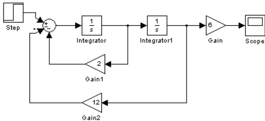
Step response for the block diagram is shown below
