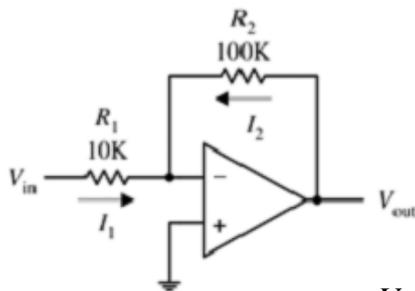
$$Gain = \frac{V_o}{V_i} = -\frac{R_2}{R_1}$$
