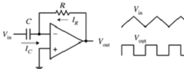
$$V_o = -RC \frac{\partial V_{in}}{\partial t}$$
