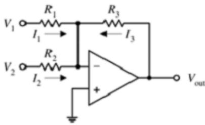
$$V_o = -\left(\frac{R_3}{R_1}V_1 + \frac{R_3}{R_2}V_2\right)$$
