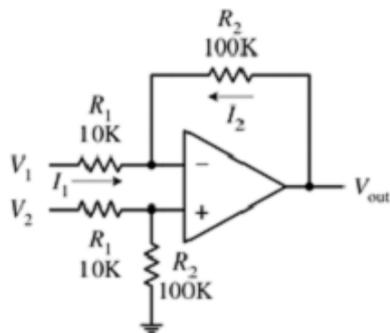
$$V_{out} = \frac{R_2}{R_1}(V_2 - V_1)$$
