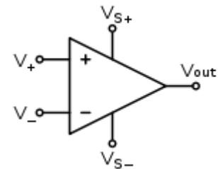
Operational amplifiers can be used to perform mathematical operations on voltage signals such as inversion, addition, subtraction, integration, differentiation, and multiplication by a constant.
