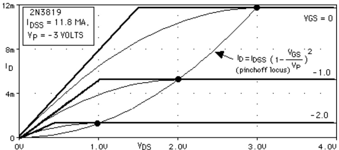
Computed drain characteristics covering both the VCR range and saturation are drawn below.
