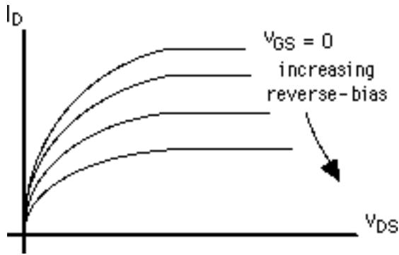
A still more extended range of variation of the drain characteristics is sketched to the right. The voltage-controlled (VCR) region, i.e., operation before pinch-off, is conventionally called (mostly) just that, i.e., VCR region. The 'constant' current (pinch-off) region to the right is 'saturation' (probably all the remarks respecting a conflict with BJT terminology already have been said, repeatedly).
