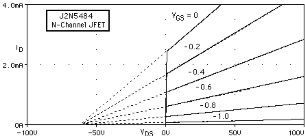
To account for this effect analytically the saturation characteristics may be multiplied by a factor  $1 + \lambda V_{DS}$ , essentially the leading terms of a series expansion:
