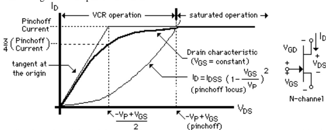
The tangent line from the origin and the saturation current provide convenient asymptotes with which to sketch a characteristic fairly accurately; note again that the actual current is 3/4 that at the intersection of the asymptotes.
