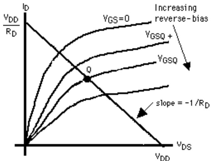
Suppose now the gate voltage is changed, say increased (i.e., made less negative) to  $V_{GS+}$ . There is a consequent increase in drain current, an increase in the voltage drop across the drain resistor, and a decrease in the drain-source voltage. Locating the new operating point graphically is a matter of moving 'up' the load line to the transistor characteristic identified by the gate voltage  $V_{GS+}$ .
