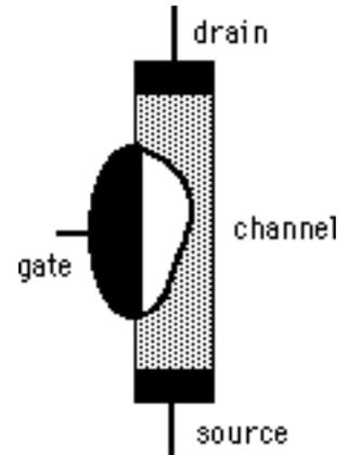
By convention the terminal designations are defined so that carriers (electrons for the N-channel device) flow from the source and to the drain. For the N-channel device, therefore, a voltage is assumed to be applied so that the drain is positive relative to the source.
