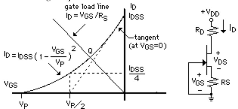
A (rough) illustrative design using the 2N5484 JFET in the circuit described above follows; the common source characteristics (Pspice model) for the 2N5484 are reproduced below.
