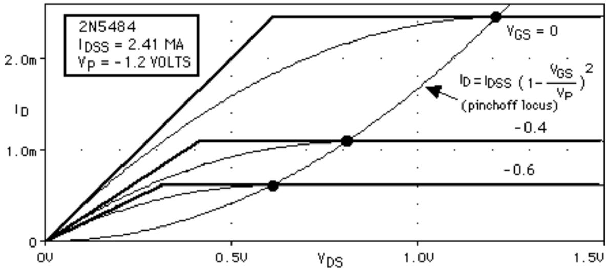
To obtain an estimate of the channel resistance in the VCR region (for small values of  $V_{DS}$ ) we can use the ratio of coordinates of the asymptote intercept point, i.e., the slope of the tangent at the origin.. For the  $V_{GS} = 0$  characteristic this estimate is  $(-V_P/2)/I_{DSS} = (1.21/2)/0.00241 = 251 \text{ } \Omega$ ; the channel resistance increases for more negative gate voltages.
