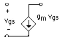
In the saturation range of operation, and neglecting second order channel-length modulation
