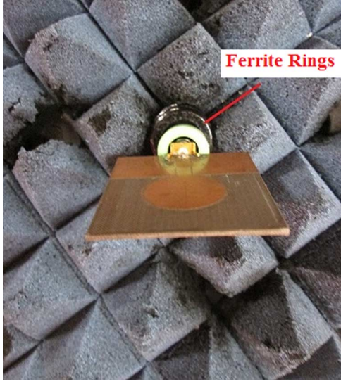
Fig. 5. Fabricated prototype mounted in the anechoic chamber with cable covered with ferrite rings.
