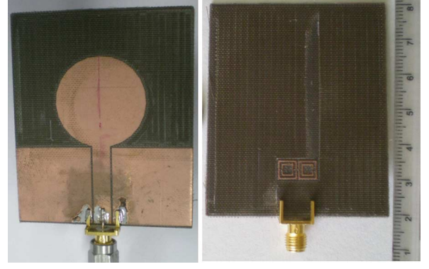
Fig. 2. Fabricated prototype of the CPW fed circular monopole loaded with SRR. Parameters as in Table I.
