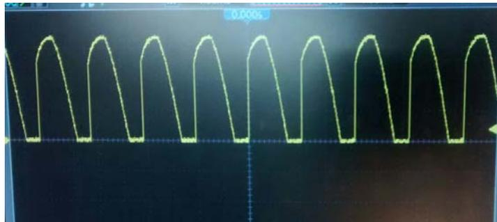
Fig. 7 Waveform of output voltage for firing angle,  $\alpha=30^\circ$
