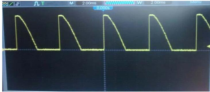
Fig. 8 Waveform of output voltage for firing angle,  $\alpha=90^\circ$
