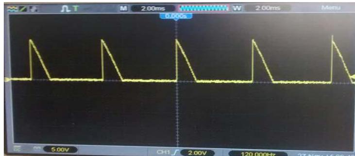
Fig. 9 Waveform of output voltage for firing angle,  $\alpha=150^\circ$
