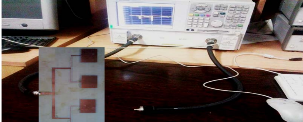
Fig. 10 Prototype fabricated antenna under testing
