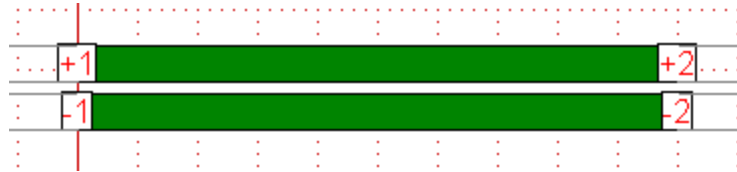
Figure 15.6 The positive and negative terminals for a symmetrical differential structure.
