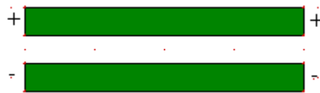
Figure 15.1 A pair of coupled strips for differential excitation.
