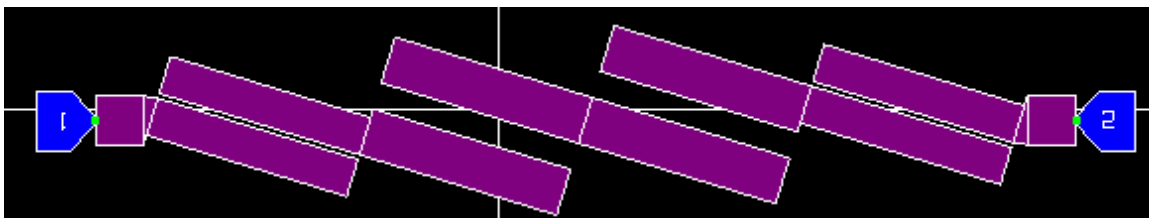
Figure 10.12 The BPF filter with 2 extension ports on it.
